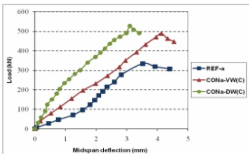
**Fig. 2.** load-deflection behavior of deep beams strengthened with CFRP sheets.
