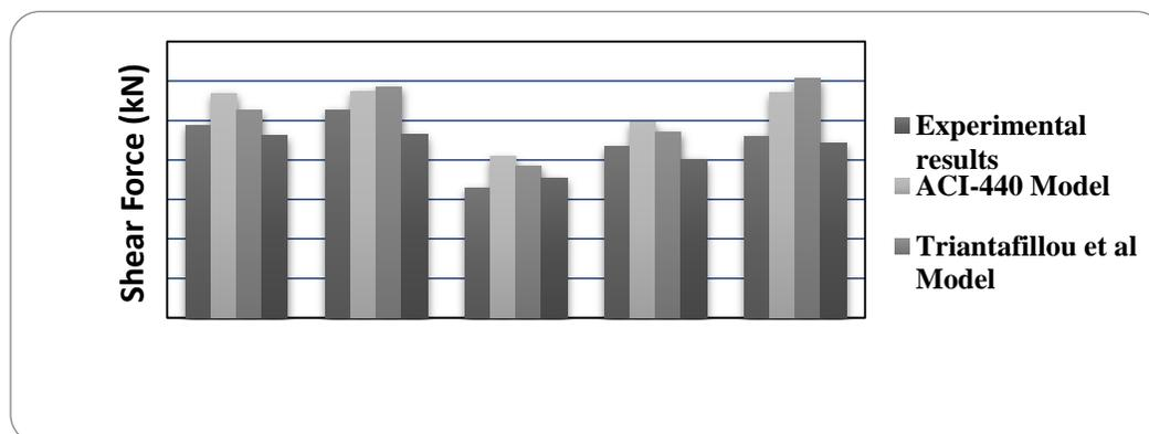
Fig. 6. Comparison of experimental results with theoretical values of strengthened beams
