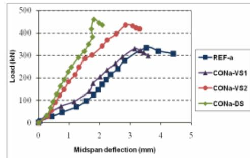
**Fig. 3.** load-deflection behavior of deep beams strengthened with CFRP Laminates
