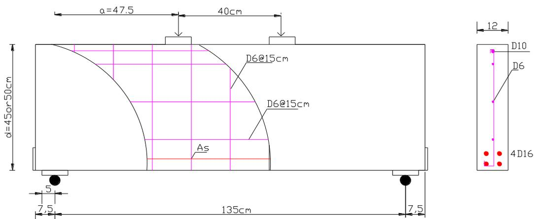
**Fig. 1.** Dimension and internal reinforcement details of reference deep beam specimen
