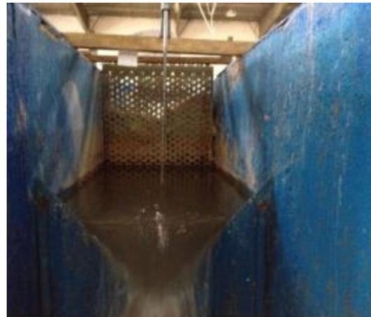
Fig. 1. Triangular weir for flow measurement
