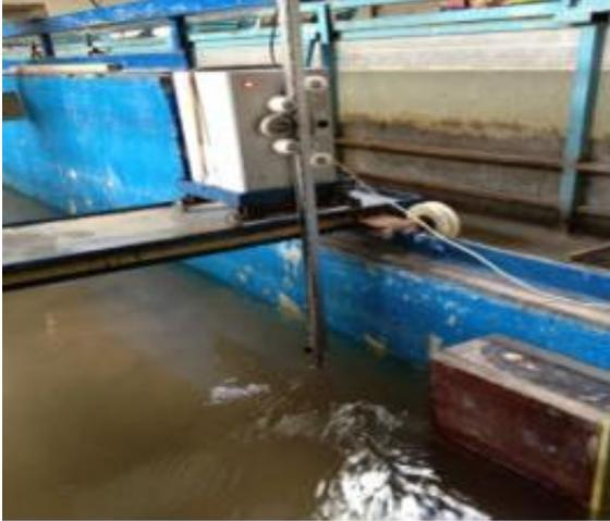
**Fig. 3.** Profiler to measure the bed depth changes
