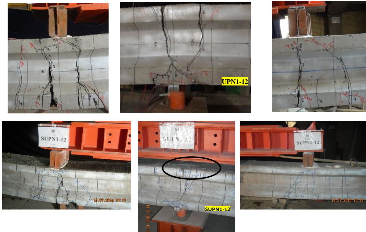
Fig. 2. Typical crack pattern of tested beams
