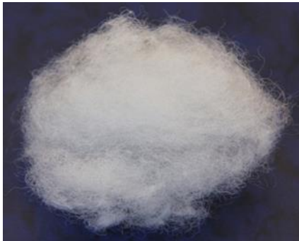
Fig. 1. Picture of recycled polyester fibers
