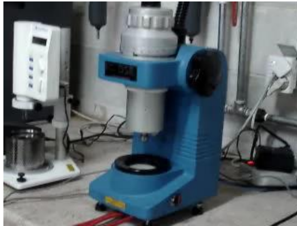
Figure 1. The DSR test apparatus
