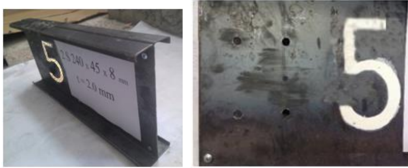
Fig. 19. Undamaged specimens after loading (elastic buckling), web elastic buckling without damage in holes.
