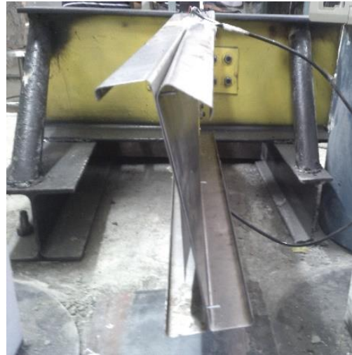
Fig. 16(b). Specimen No.3 subjected to the gravity load.
