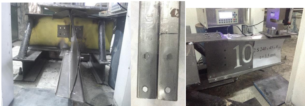
Fig. 21. Web plastic buckling without considerable damage in flanges and holes.
