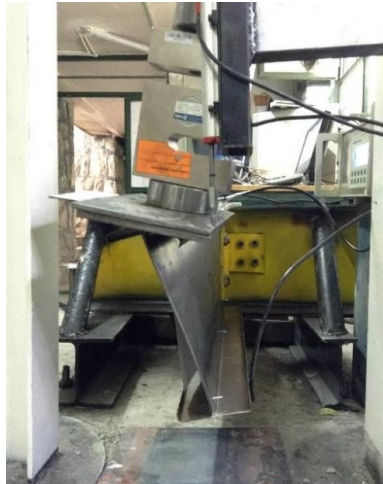
Fig. 16(a). After loading (plastic buckling).
