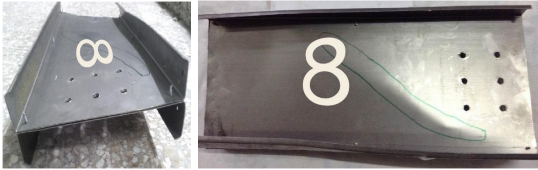
Fig. 13. Deformation mechanism of test specimen No. 8.
