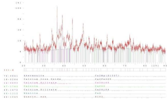
Figure 1- XRD Spectrum result of the tested steel slag
