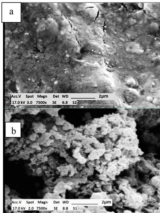
**Figure 2.** Morphological characteristics of aggregates from SEM photos (a: limestone aggregate, b: slag aggregate)
