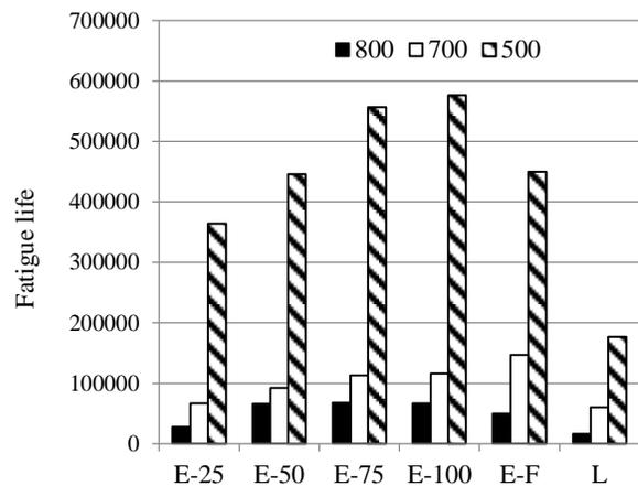
Figure 5. Fatigue life of specimens based on Pronk and Hopman method (Strain control)
