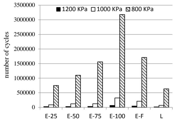
**Figure 9.** Fatigue life of specimens based on Pronk and Hopman method (Stress control)
