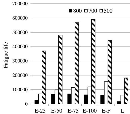
Figure 4. Fatigue life of specimens based on Rowe and Bouldin method (Strain control)
