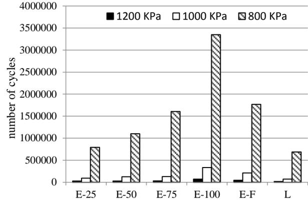
**Figure 8.** Fatigue life of specimens based on Rowe and Bouldin method (Stress control)
