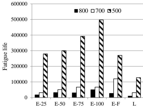
**Figure 6.** Fatigue life of specimens based on 50% stiffness reduction method (Strain control)
