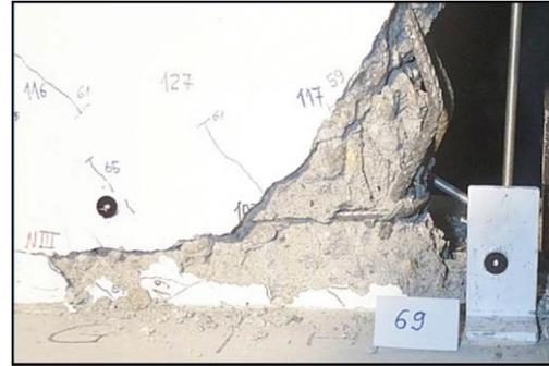
**Figure 1.** Experimental specimen M3 shear wall [18]
