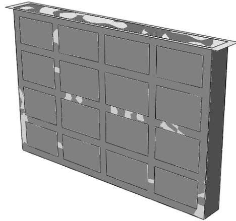
**Figure 5.** Concrete shear wall with Chess Layers
