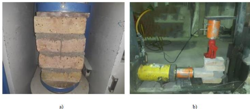
Fig. 2. Experimental tests: a) Compression and b) Shear tests on masonry specimens.
