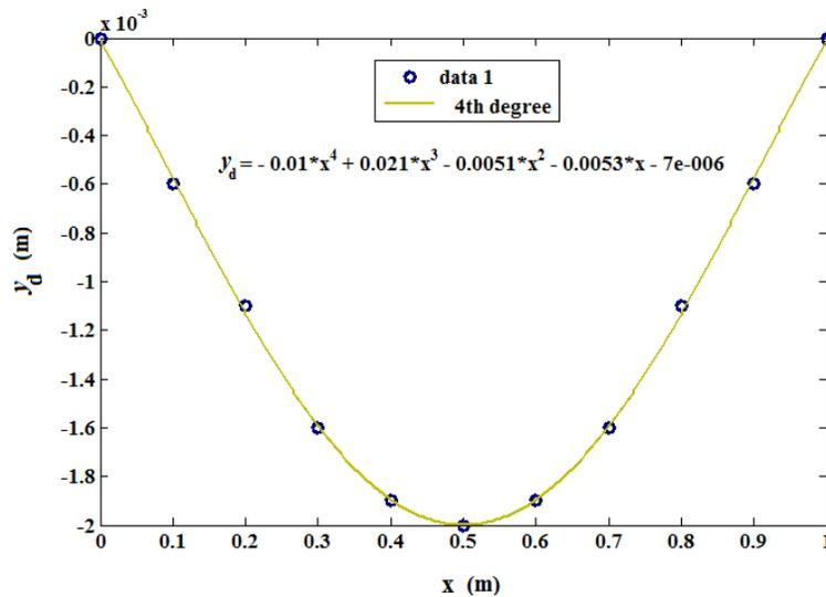
Fig. 7. Deformed shape and deflection equation of the simply supported damaged beam
