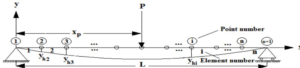
Fig. 2. Displacements of the simply supported intact beam under a concentrated load
