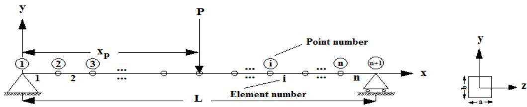
Fig. 1. (a) The geometry of the simply supported intact beam (b) Cross-section of the beam
