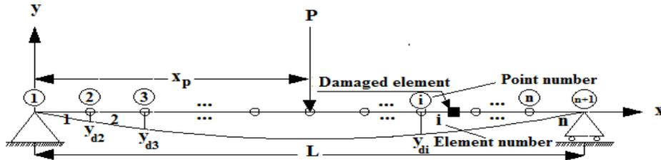
Fig. 3. Displacement of the simply supported damaged beam under a concentrated load
