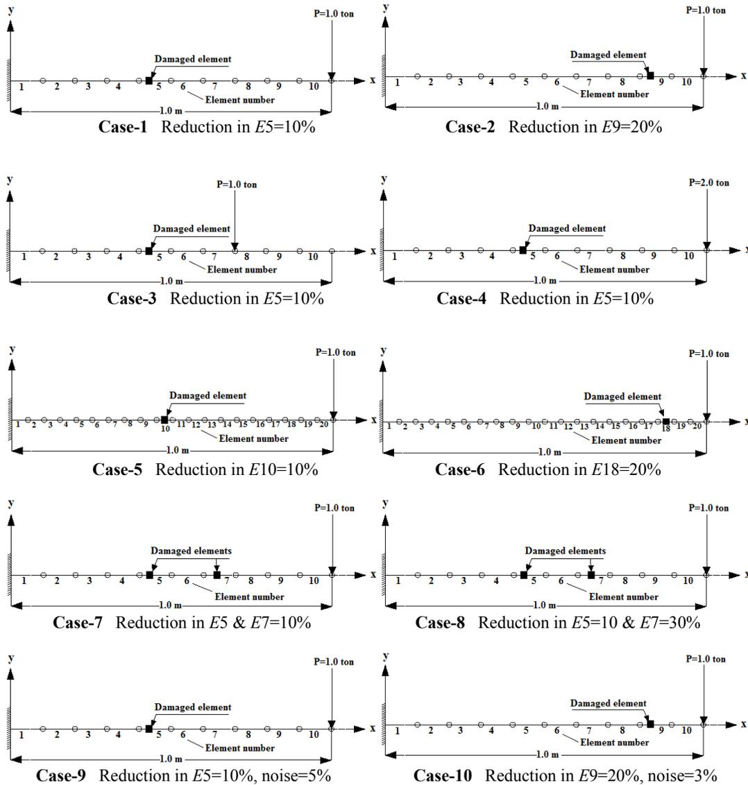
Fig. 10. Ten different damage scenarios for the cantilever beam
