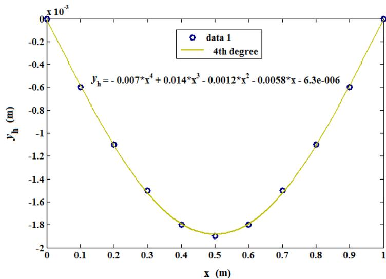
Fig. 6. Deformed shape and deflection equation of the simply supported intact beam
