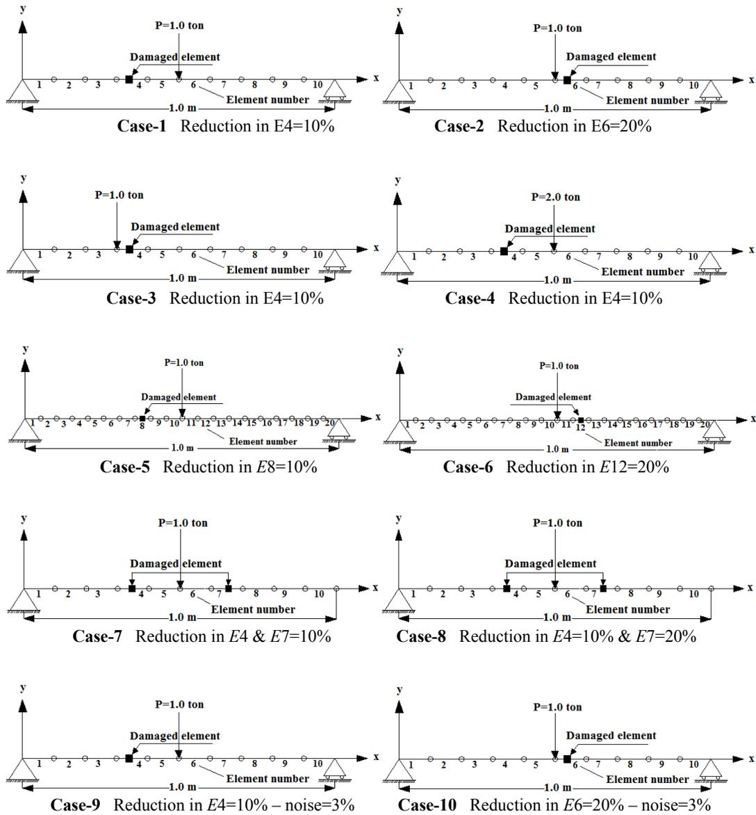
Fig. 5. Ten different damage scenarios for the simply supported beam
