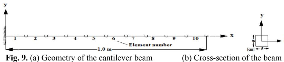
Fig. 9. (a) Geometry of the cantilever beam (b) Cross-section of the beam
