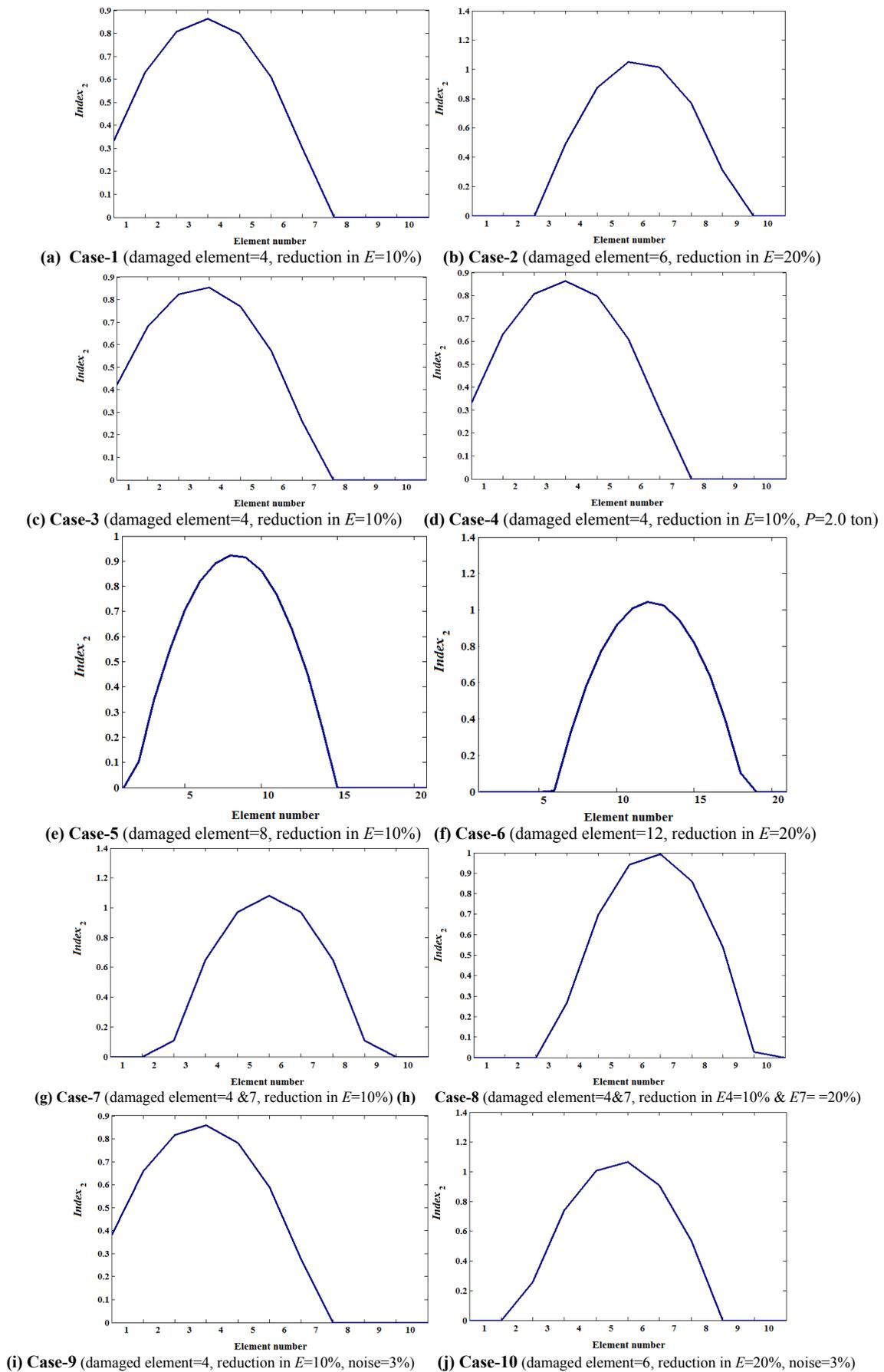
Fig. 8. Damage identification of simply supported beam for cases 1-10
