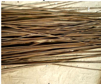
Fig. 6. Improper maintenance of material (bars)
