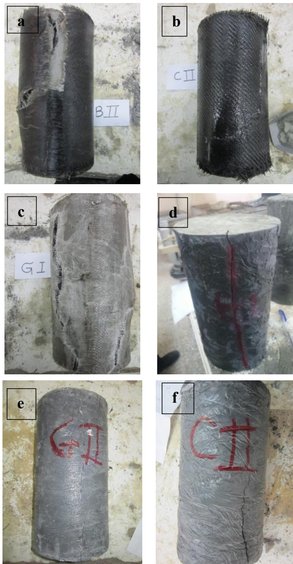
Fig.8. Failure modes of wrapped- concrete cylinders with: Organic matrix, (a) Basalt, (b) Carbon, (c) Glass and Inorganic, (d) Basalt, (e), Glass, (f) Carbon.
