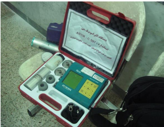
Figure 2: Ultrasonic device and Schmidt hammer
