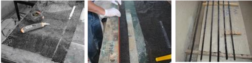
Fig. 3. Making the process of hand-made CFRP bars.
