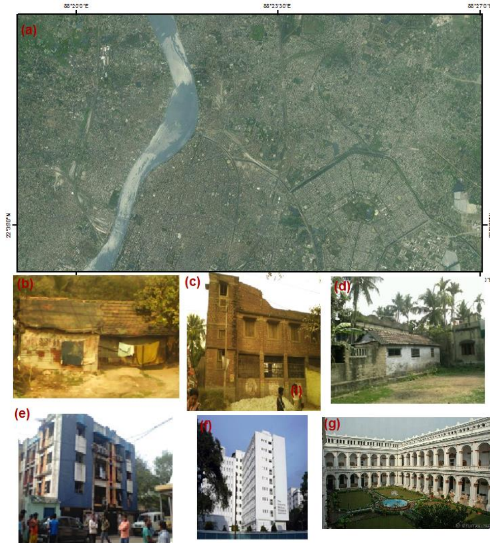
Fig. 3. The city of Kolkata accomplished with (a) Dense Built environment extracted from Google Earth and different building types viz. , (b) A1, (c) RS2 (d) URM (e) C1 (f) C3, & (g) HER (Indian Museum located at Chowringhee: Lat : 22° 33' 29" N, Long : 88° 21' 3" E).
