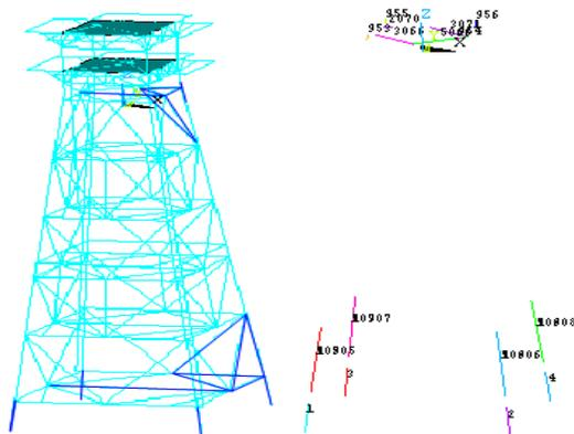
**Fig. 3.** The more critical members of the jacket structure identified by POA.
