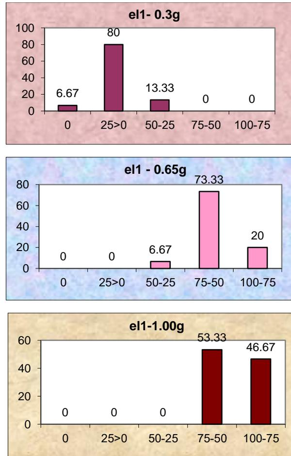
**Fig. 5.** Damage percent of element No. 1 for various PGA levels in NLTHA
