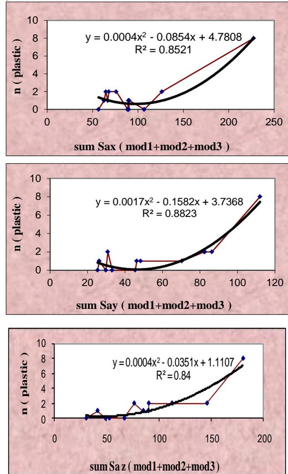
**Fig. 9.** Correlation between damage index and  $S_{a1}+S_{a2}+S_{a3}$ .
