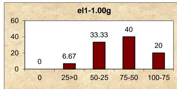
Fig. 6. Rupture percent of element No. 1 for various PGA levels in NLTHA.
