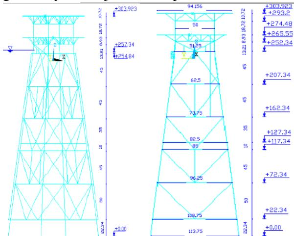
Fig. 1. The geometric features of the jacket structure.
