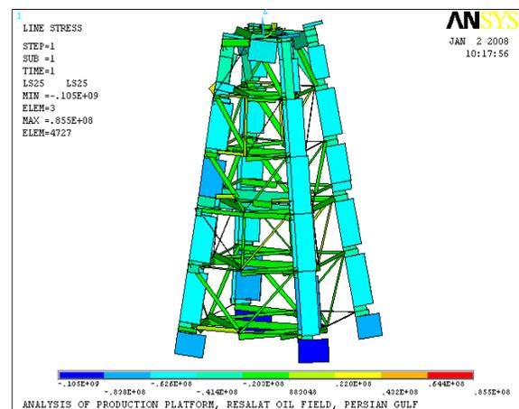
**Fig. 4.** Diagram of normal stress values in the jacket legs due to vertical loads.
