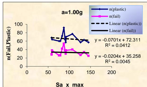
Fig. 8. The relation between the spectral response of acceleration and the number of locations with plastic and failure deformations.
