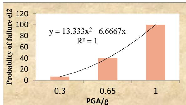
Fig. 7. Probability of failure in element No. 2 for various PGA levels in NLTHA.
