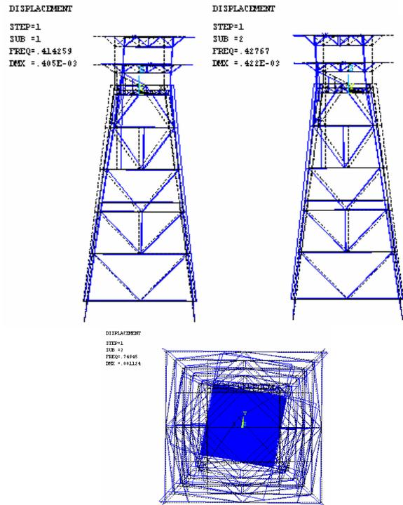
Fig. 2. Modal shapes of the first three modes of the jacket structure.
