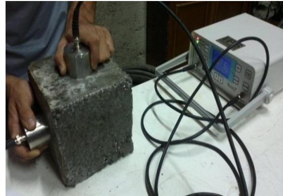
Fig. 2. Velocity test for indirect transmission of pulses.
