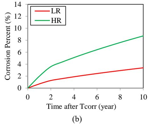
Fig. 1. Corrosion percentage of longitudinal and horizontal bars over time; (a) No Repair, (b) using shotcrete. (w/c=0.35).
