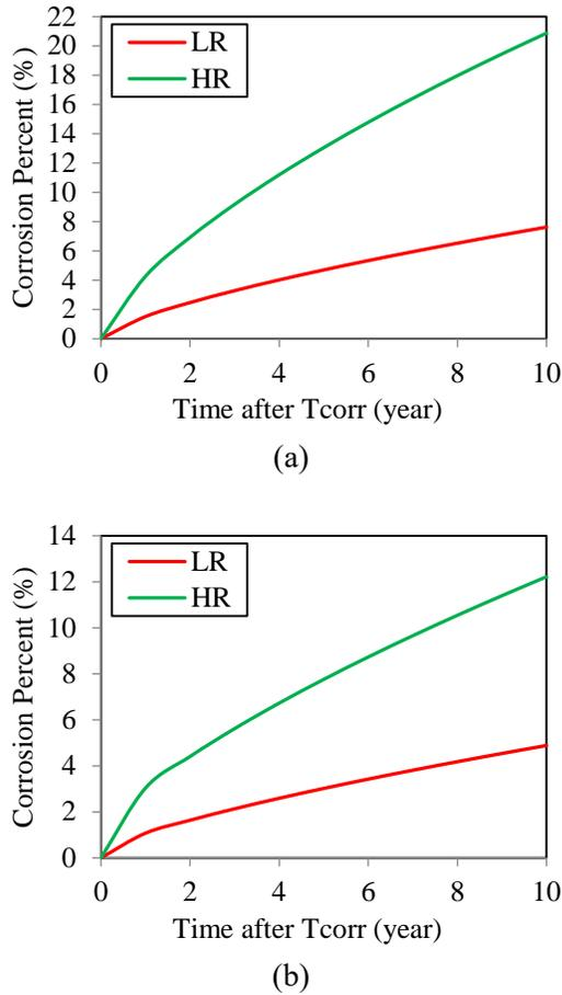
**Fig. 3.** Corrosion percentage of longitudinal and horizontal bars over time; (a) No Repair, (b) using shotcrete. ( $w/c=0.50$ ).
