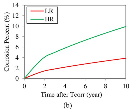
Fig. 2. Corrosion percentage of longitudinal and horizontal bars over time; (a) No Repair, (b) using shotcrete. (w/c=0.40).
