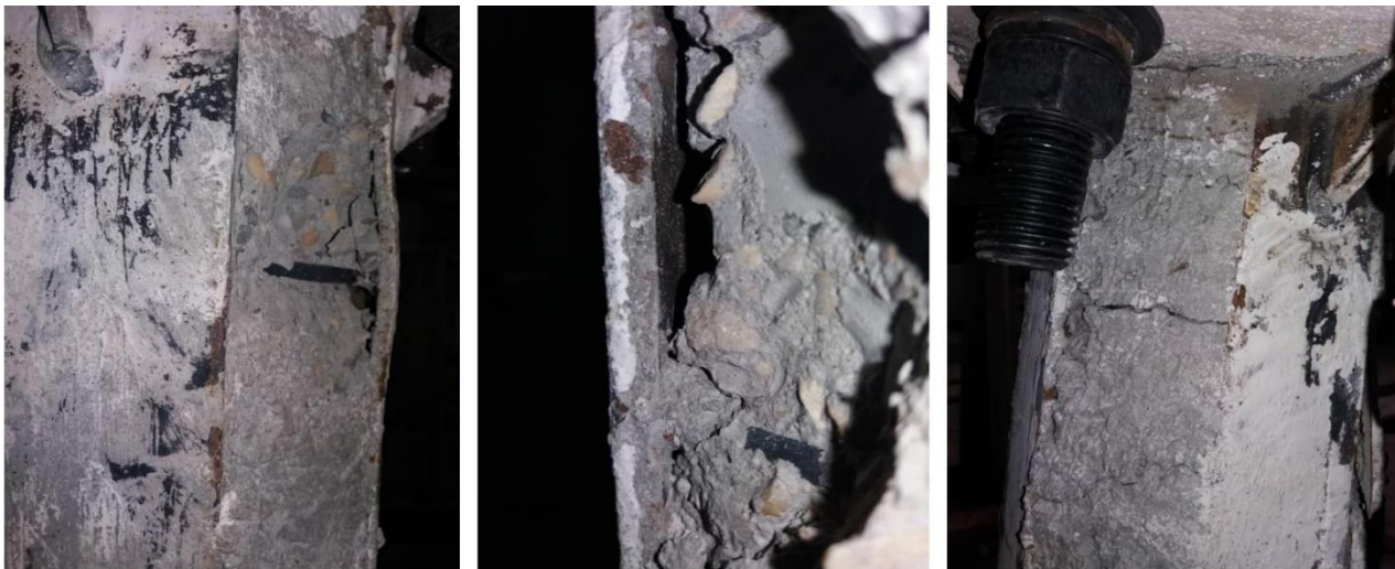
Fig. 9. Final stage of columns under bending loading, (a)PEC-1, (b)PEC-2, (c)PEC-3.
