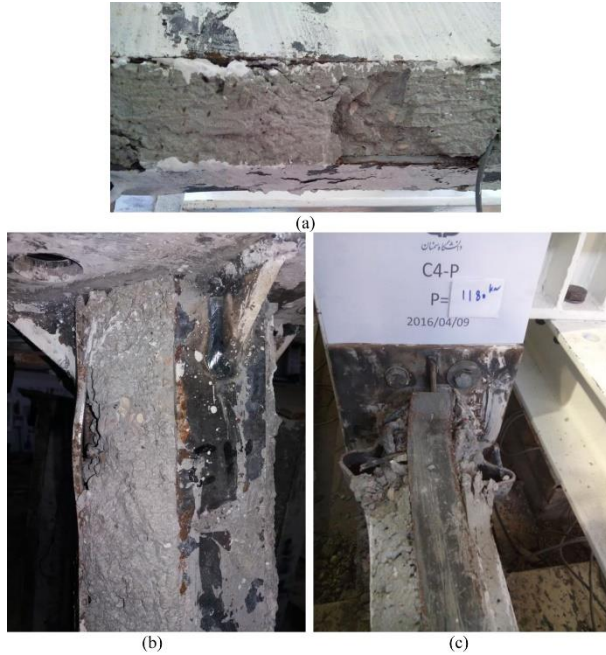
Fig. 5. Buckling of flanges, crushing concrete, and fracturing in samples: (a) PEC-1, (b) PEC-2, (c) PEC-3.
