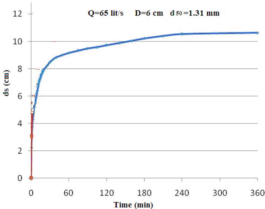
**Fig. 3.** Comparison between time variations of depth of local scour in front of the first pier
