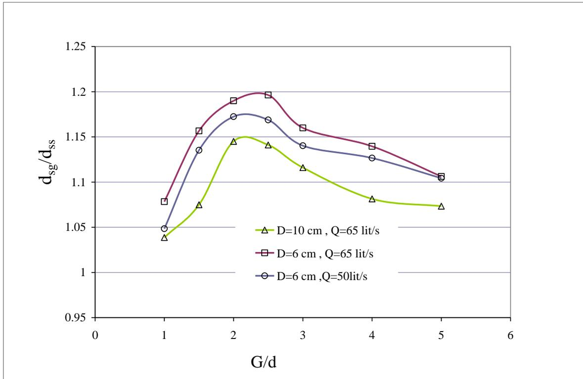
**Fig. 4.** Variations of  $d_{sf}/d_{ss}$  relation to variations of  $G/D$  (cylindrical group pier and  $d_{50}=1.31$  mm)
