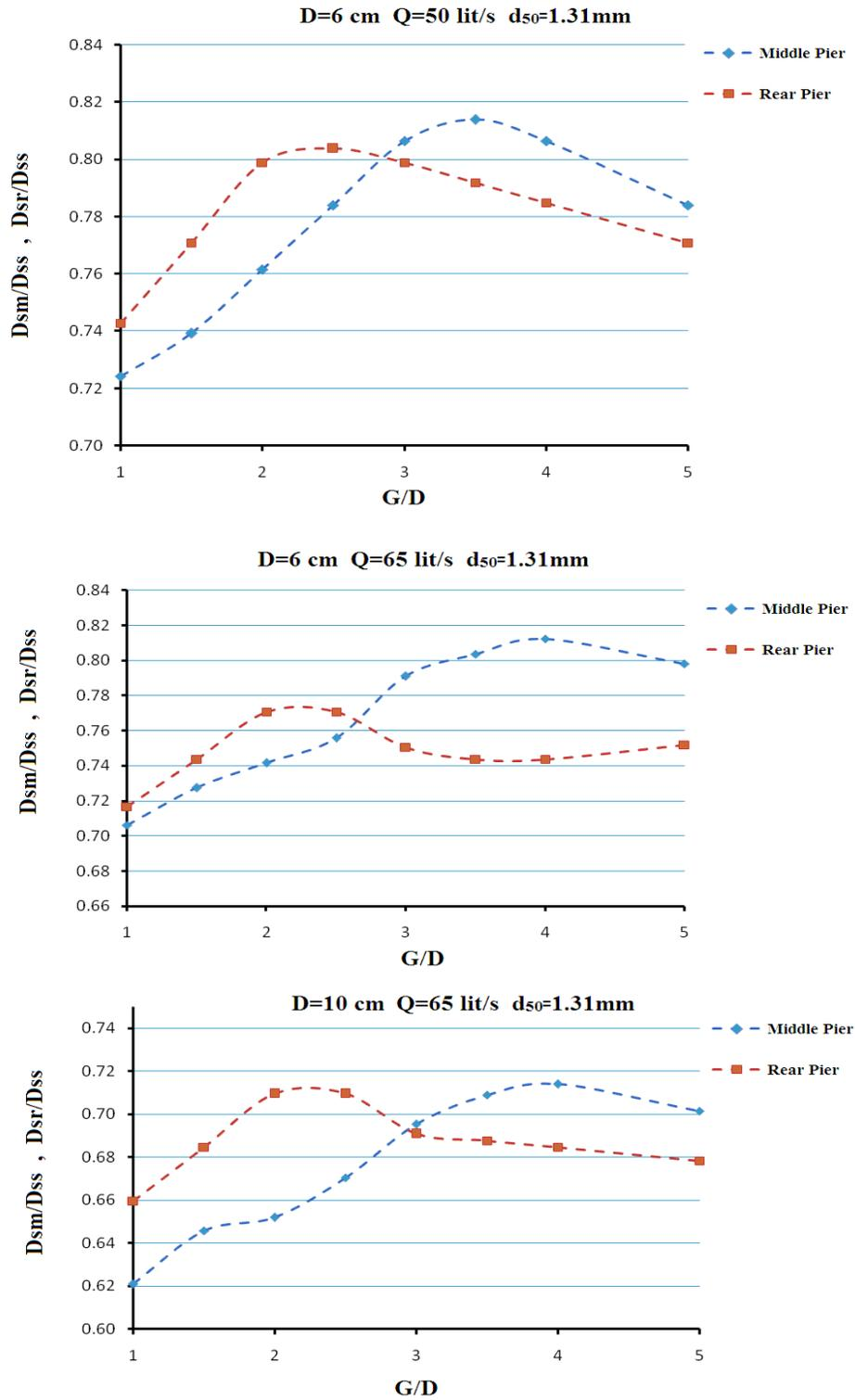
Fig. 5. Comparison between  $D_{Sm}/D_{Sf}$  and  $D_{Sr}/D_{Sf}$  for different  $G/D$ s and tests
