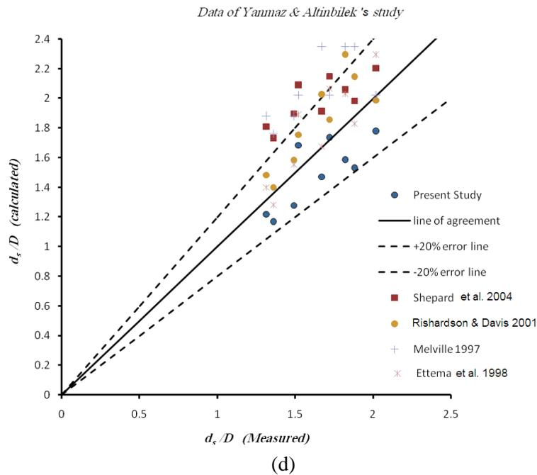
**Fig. 6.** a) Comparison between results of this study and Sheppard et al. [16] equation (Data of Sheppard et al. [34]) b) Comparison between results available equations c) Comparison between results of this study and other equations (Data of Sheppard et al. [34]) d) Comparison between results of this study and other equations (Data of Yanmaz and Altinbilek [8])
