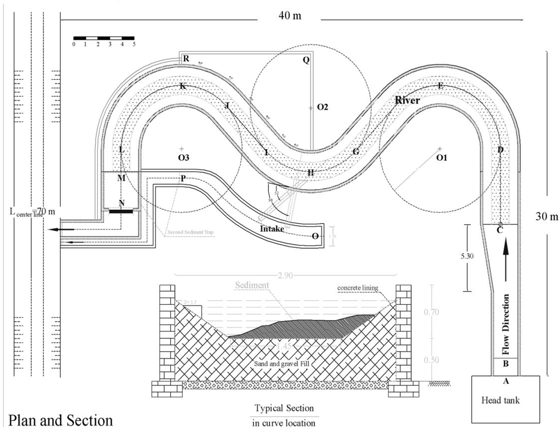
**Fig. 1.** The plan and section of constructed experimental flume.
