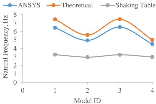
Fig. 5. Natural frequency of models obtained from different analysis.
