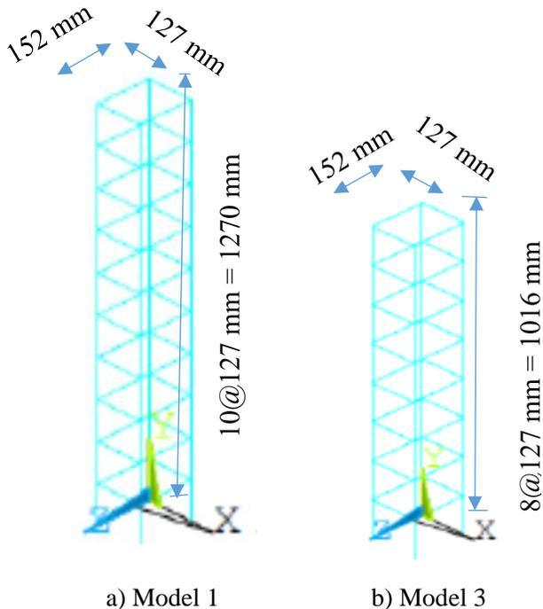
Fig. 2. Structural models.
