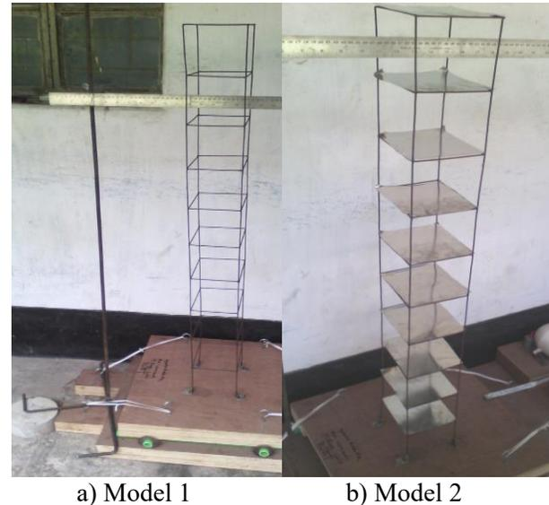
Fig. 3. Models under shaking table test.
