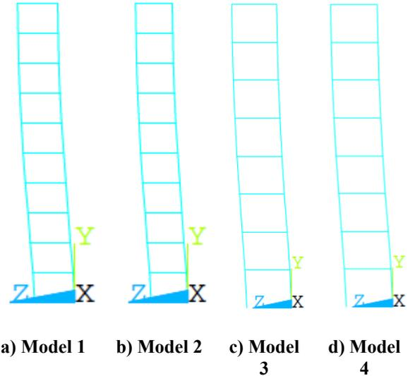
**Fig. 4** 1<sup>st</sup> mode shape of structural models.
