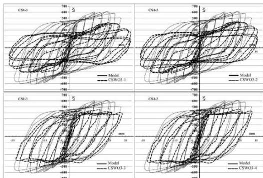
**Fig. 8.** The load-displacement curve of experimental specimen CS1-3 without opening vs. the four experimental developed specimens containing opening.
