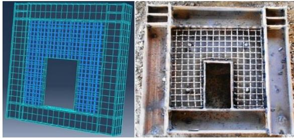
**Fig. 9.** the developed ABAQUS model and the experimental specimen before loading (csw03).
