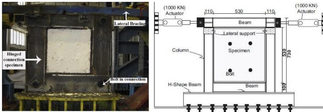
Fig. 1. Arabzadeh et al. specimen before loading and the test setup [3].
