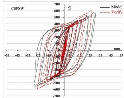
Fig. 3. Load-displacement hysteresis curves of reference specimen and Arabzadeh et al. specimen.
