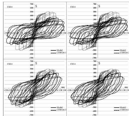
**Fig. 13.** The experimental load-displacement curves of specimen CS3-1 without opening [10] vs. the four experimental models with opening.
