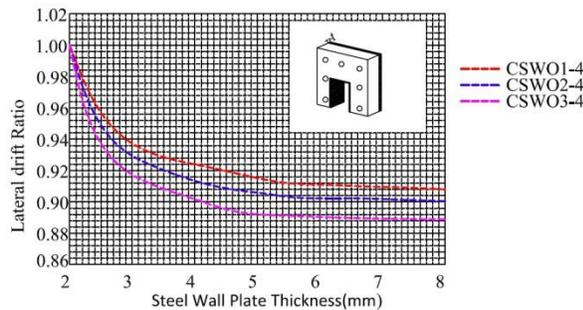
**Fig. 17.** Effect of thickness of infill steel plate on drift ratio.
