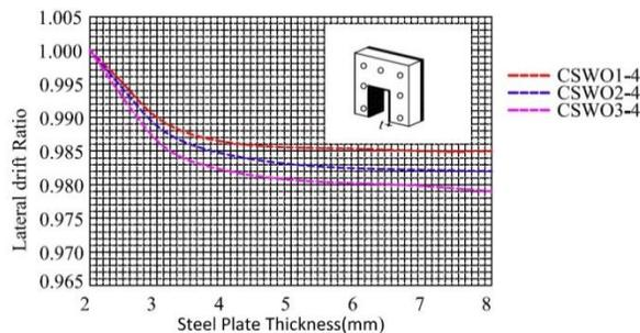
**Fig. 18.** Effect of thickness of strengthening steel plate on drift ratio.
