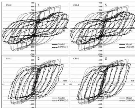
**Fig. 7.** The load-displacement curve of experimental specimen CS1-2 without opening vs. the four experimental specimens containing opening.
