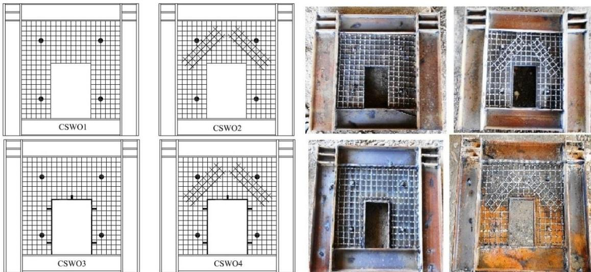
Fig. 4. The developed models for CSPSWs with opening.
