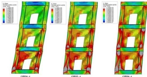
**Fig. 11.** Deformed shape of the second series of specimens after numerical analysis.
