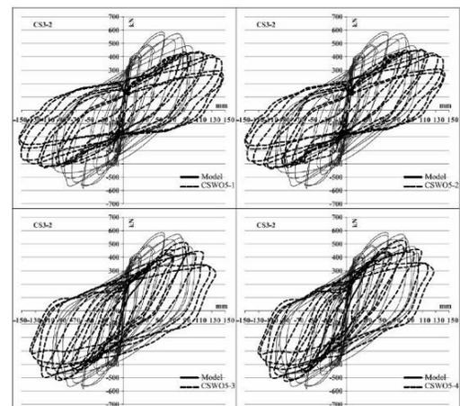
**Fig. 14.** The experimental load-displacement curves of specimen CS3-2 without opening [10] vs. the four experimental models with opening.
