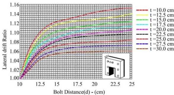
**Fig. 16.** Effect of bolt distances and concrete panel thickness on drift ratio.
