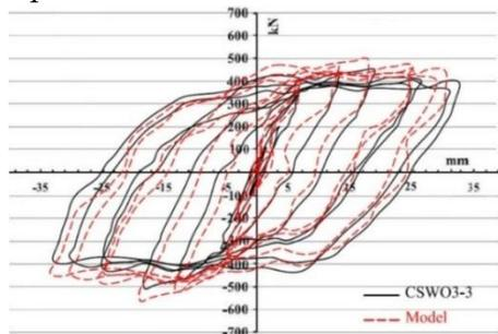
**Fig. 10.** Experimental vs. numerical load-displacement hysteresis curves.
