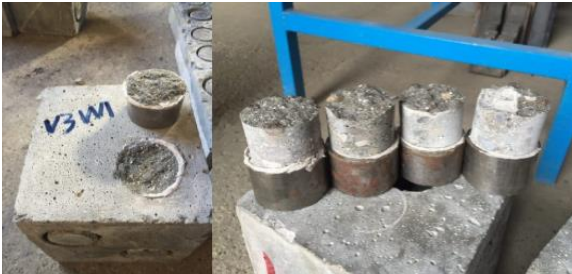
Fig. 3. Failure surfaces in Pull-off test on 15cm cubes (left: without coring, right: with coring).
