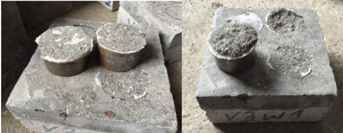
Fig. 2. determination of in-situ strength of repair layer using Pull-Off (without coring).
