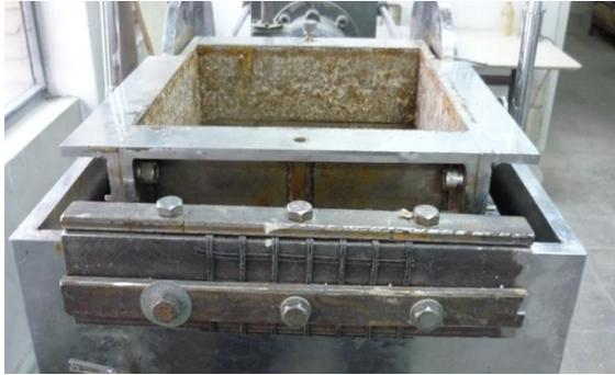
Fig. 4. Connection of geogrid with outer box.
