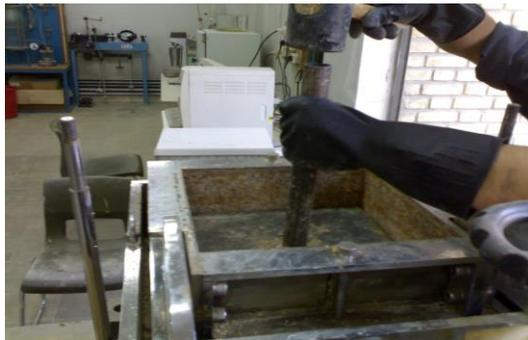
(b) Compacting layer of soil in shear box.
