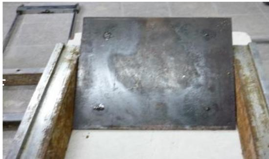
(a) Steel plate under the shear box.
