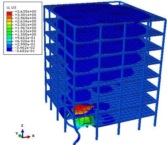
Fig. 16. Vertical displacement contour (case1)
