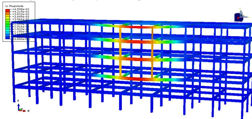
Fig. 7. Displacement of the OHIO building after removing two columns (With the finite element method of this study)
