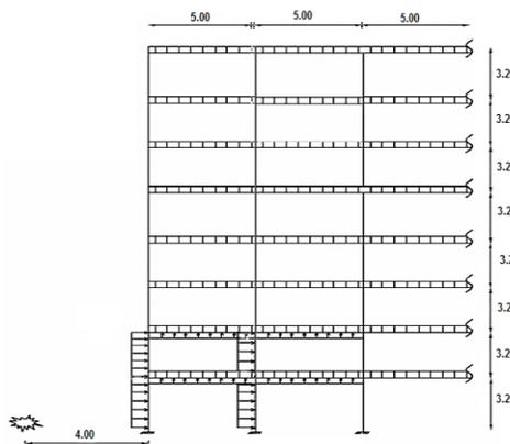
Fig. 14. The manner of applying the blast load on the given structure components (e.g., case4)
