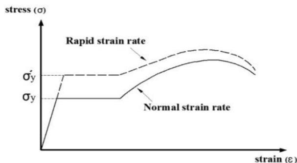
Fig.4. The Diagram of Strength Increase Factor [16]
