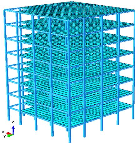
Fig. 3. 3D finite element model of the building
