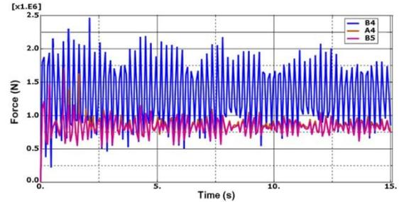
**Fig. 32.** Axial force of columns (APM method)
