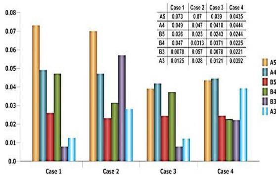
Fig. 28. Bending DCR values in different load cases
