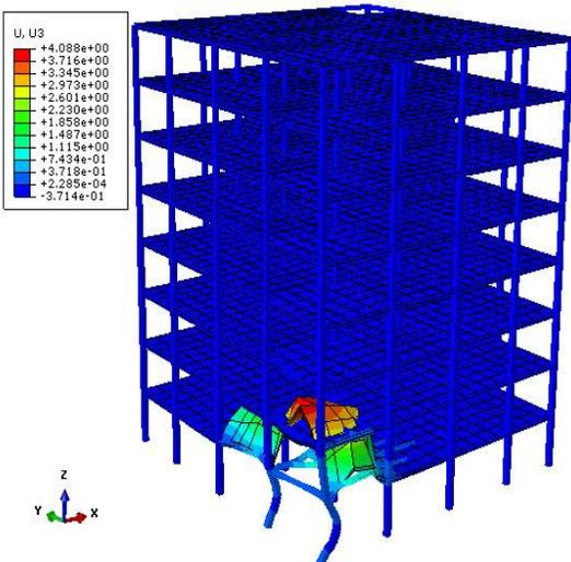
Fig. 20. Vertical displacement contour (case2)
