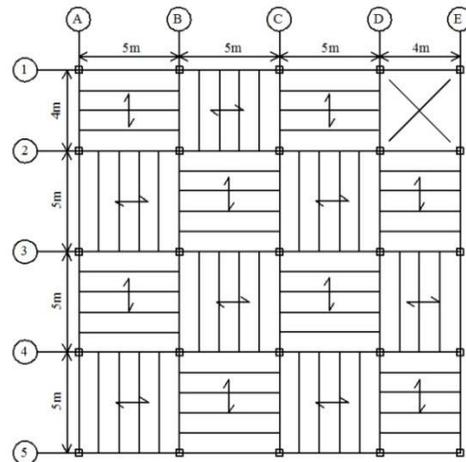
**Fig. 1.** Typical plan of 7-story prototype building
