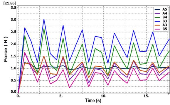
Fig. 21. Axial force of columns (case3)
