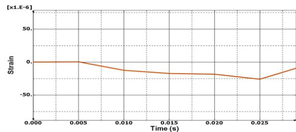
Fig. 9. Strain gauge (Number 15) measurements during column removals
