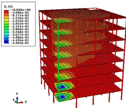
**Fig. 30.** Vertical displacement of building (APM method)
