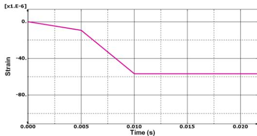
Fig. 8. Strain gauge (Number 2) measurements during column removals
