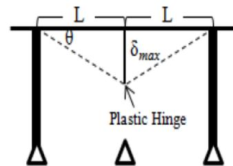
Fig. 29. Measurement of plastic hinge rotation
