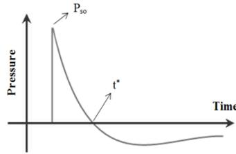
Fig. 12. Time history of the blast loading in a given time-pressure graph for slab 1
