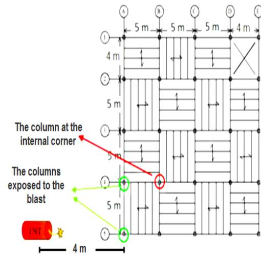
**Fig. 33.** The key member in the design of the building against progressive collapse due to blast
