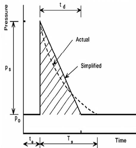
**Fig. 11.** Simplified blast-wave overpressure profile with impulse by Yandizo et al. (1999) [21]
