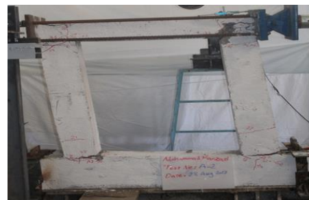
Fig. 10. RC frame at the end of loading.
