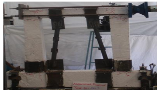
Fig. 18. EBF at the end of loading.
