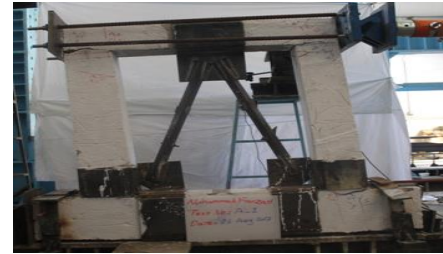
Fig. 14. CBF specimen at the end of loading.
