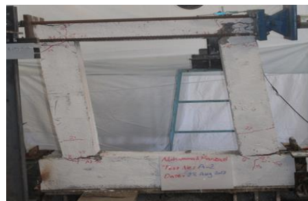
Fig. 10. RC frame at the end of loading.
