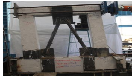
Fig. 14. CBF specimen at the end of loading.
