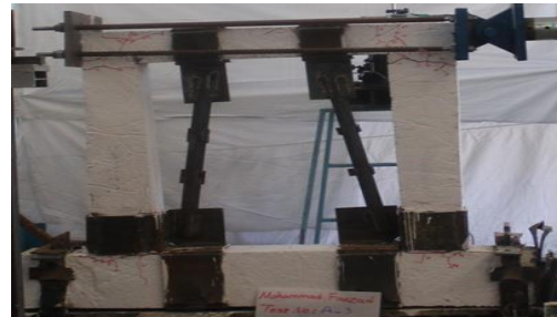
Fig. 18. EBF at the end of loading.
