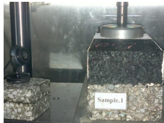
Fig. 3. Test specimen under loading in UTM-25 dynamic testing machine.
