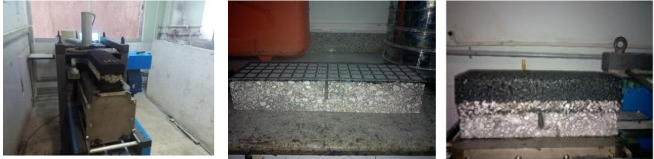
Fig. 2. The sample beam constructed by PReSBox Compactor.
