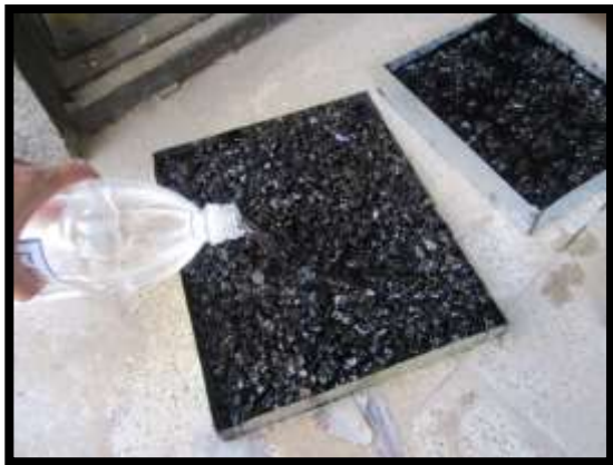
Fig. 18. Use of electrolyzed water to absorb environmental contaminants at the pavement surface.
