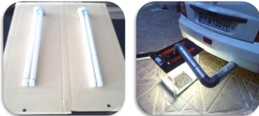
Fig. 16. Simulation of vehicle exhaust fumes at emission stage of pollutants on asphalt samples and UV light used.
