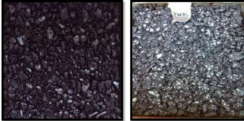
Fig. 15. Image of asphalt sample containing contamination absorbent coating with modified emulsion asphalt binder.
