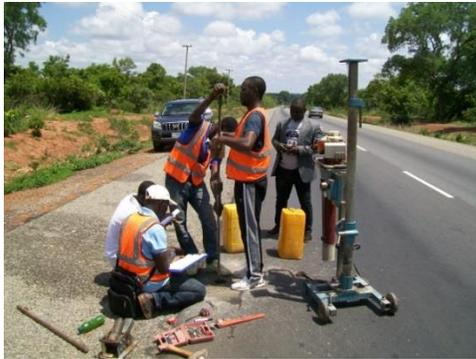
Fig. 4. Dynamic Cone Penetration test.
