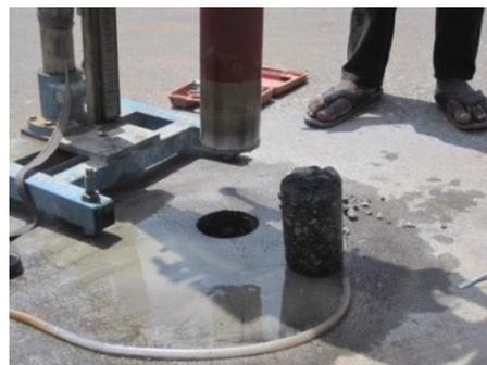
**Fig. 3.** Collection of core samples of asphalt.
