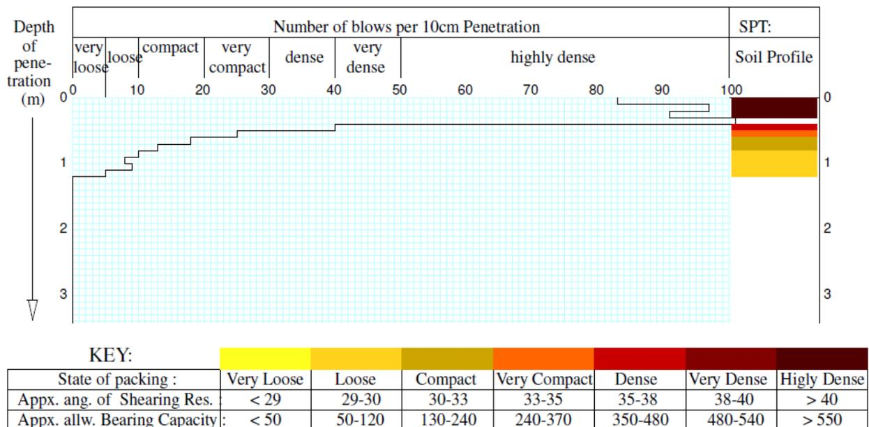
Fig. 5. DCPT Result for test location one (CH 18+600).
