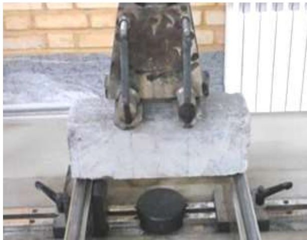
Fig. 10. Test setup of flexural specimens.
