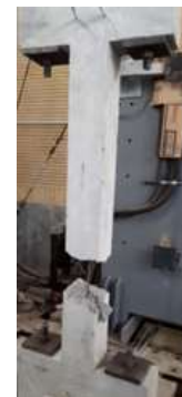
Fig. 5. Test results for specimens under monotonic loading, a) load-deflection, b) deformed rebar cracking pattern, c) plain rebar cracking pattern.
