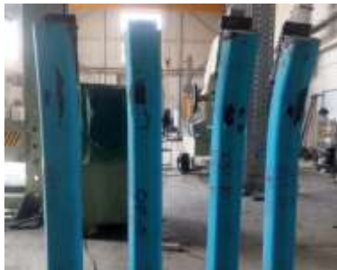
Fig. 14. Failing mode of specimens filled with plain concrete.
