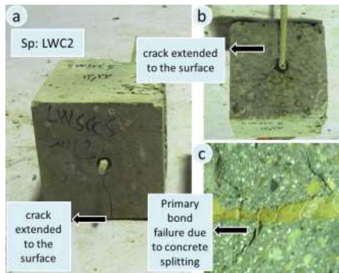
**Fig. 14.** a) Extended crack on the bottom surface b) extended crack on the top surface c) primary cracks due to the bar slippage and lack of enough shear strength.
