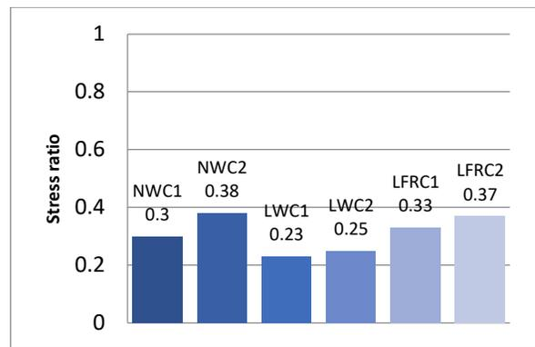
Fig. 10. Maximum tensile stress ratio developed in GFRP bar cross-section.
