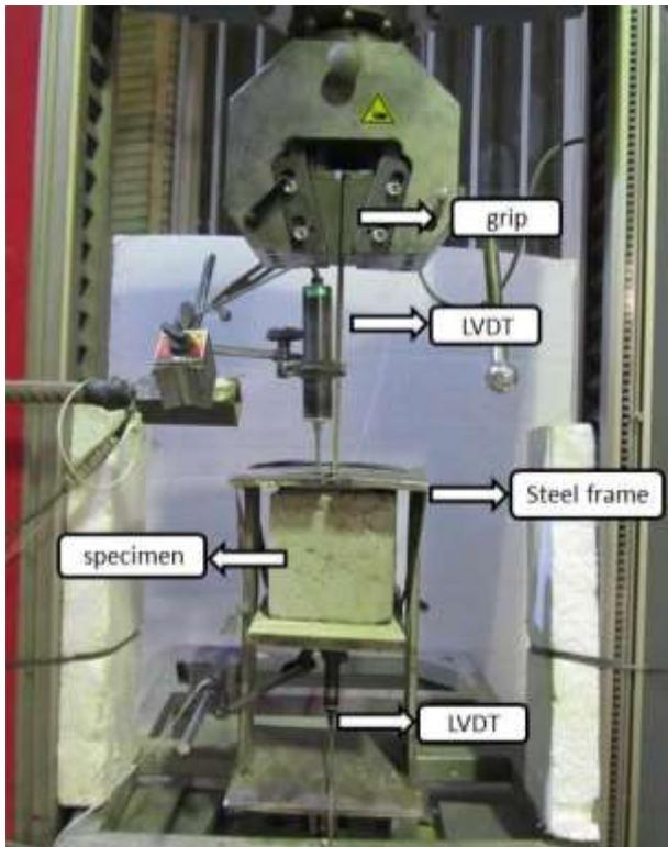
Fig. 6. Test setup and configuration.
