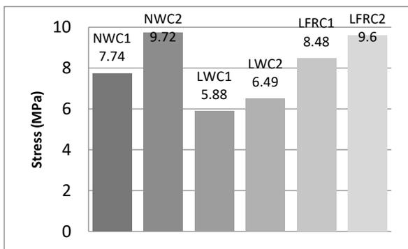
Fig. 8. Maximum bond strength in specimens.
