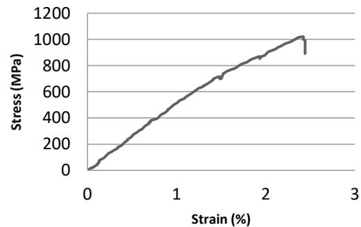
Fig. 4. Stress-strain curve of GFRP bar.
