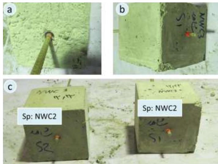
Fig. 12. a) No crack observation on the top surface b) No crack observation on the side surfaces c) Free end slippage occurs.
