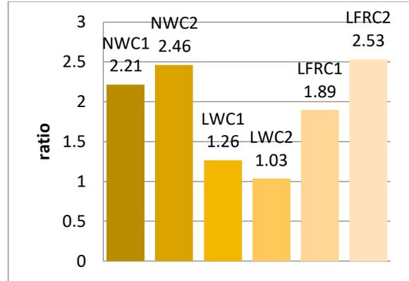
Fig. 18. The ratio of the development length proposed by ACI440.1R-15 [46] to the experimental development length.
