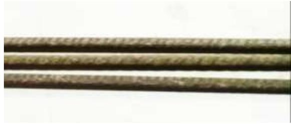
Fig. 3. Sand-coated GFRP bar.
