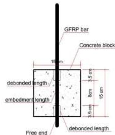
**Fig. 2.** The placement of GFRP bar embedded in concrete.
