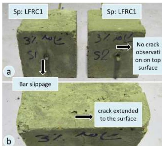
**Fig. 15.** Bar slippage occurred for specimen LFRC1.
