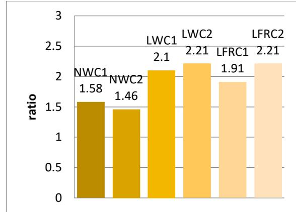
**Fig. 19.** The ratio of the development length proposed by CSA-S806-12 [47] to the experimental development length.
