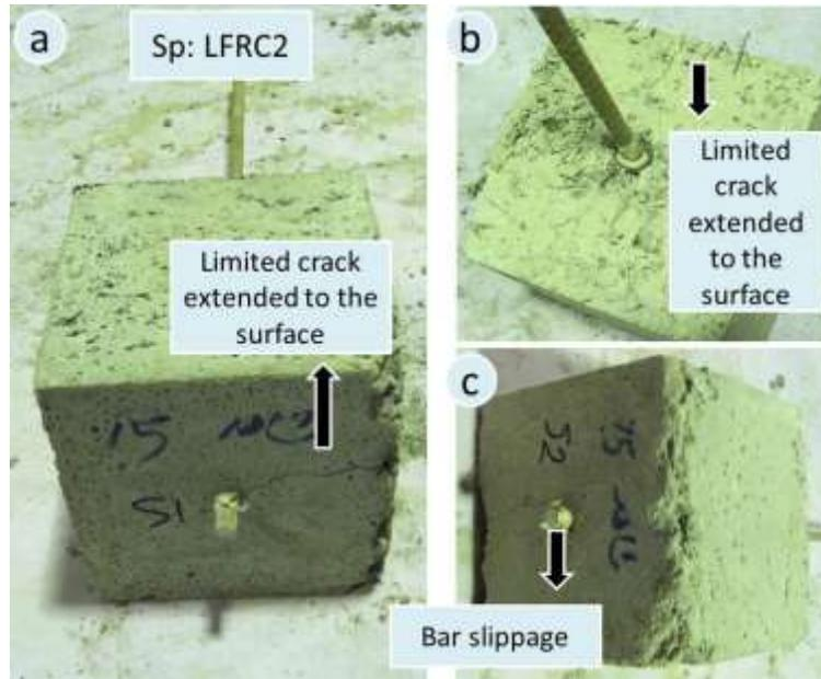
Fig. 16. Bar slippage occurs for specimen LFRC2.
