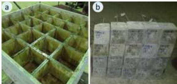
**Fig. 1.** a) Casting molds b) Prepared samples for direct pull-out test.
