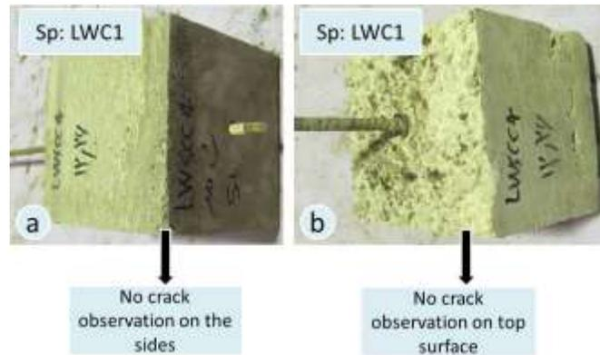
**Fig. 13.** a) No crack observation on the side surfaces b) No extended crack observation on the top surface during the bar slippage.
