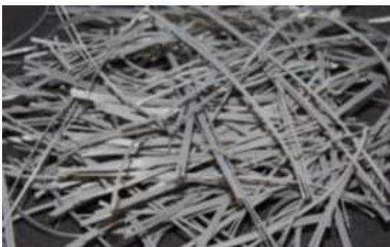
Fig. 5. Emboss macro-synthetic fiber used in LFRC1 and LFRC2.
