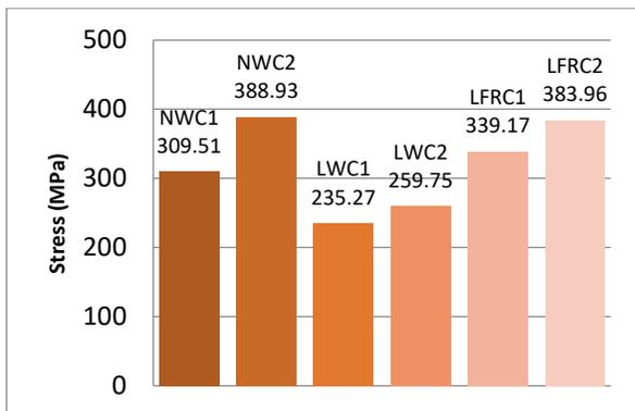
Fig. 9. Maximum tensile stress developed in GFRP bar cross section.
