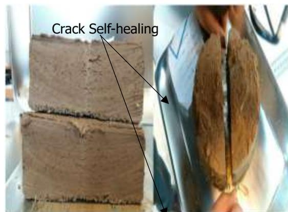
**Fig. 4.** Crack creation (right) and self-healing process of cracks (left)
