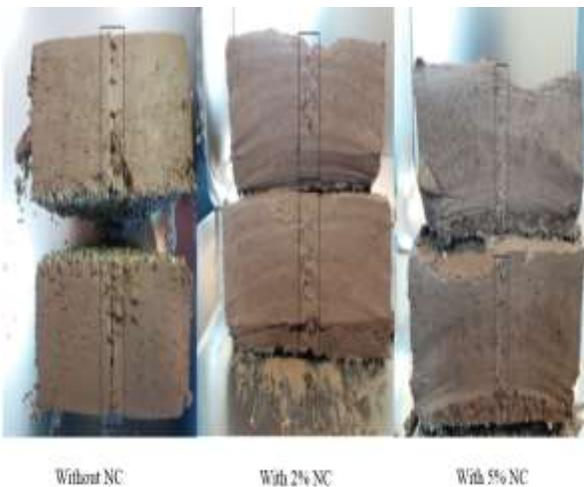
**Fig. 18.** Self-healing of samples with 1 mm crack [without pressure] (After construction)
