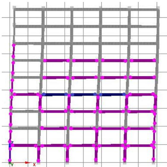
Fig. 8. IO (purple) and LS (blue) hinges of the 9-story structure.
