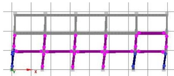
**Fig. 6.** IO (purple) and LS (blue) hinges of the 3-story structure.
