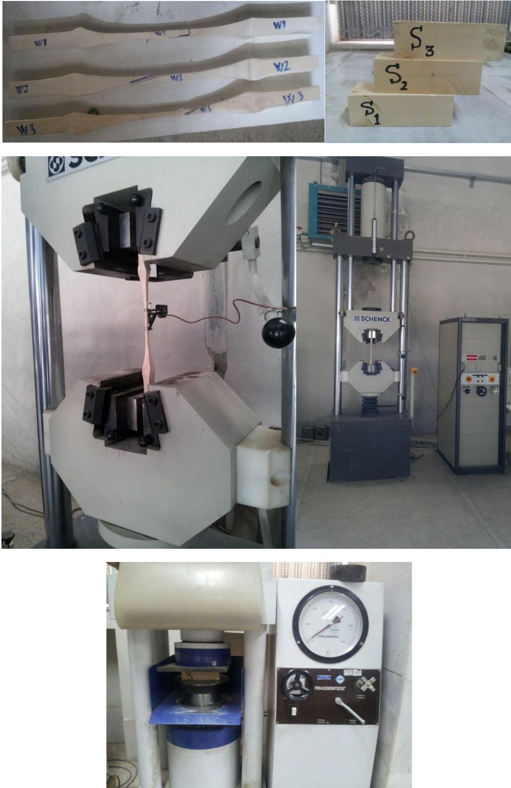
Fig. 2. Tensile and compressive specimens under Tension Parallel to Timber Grain Test and Compression Perpendicular to Timber Grain Test.
