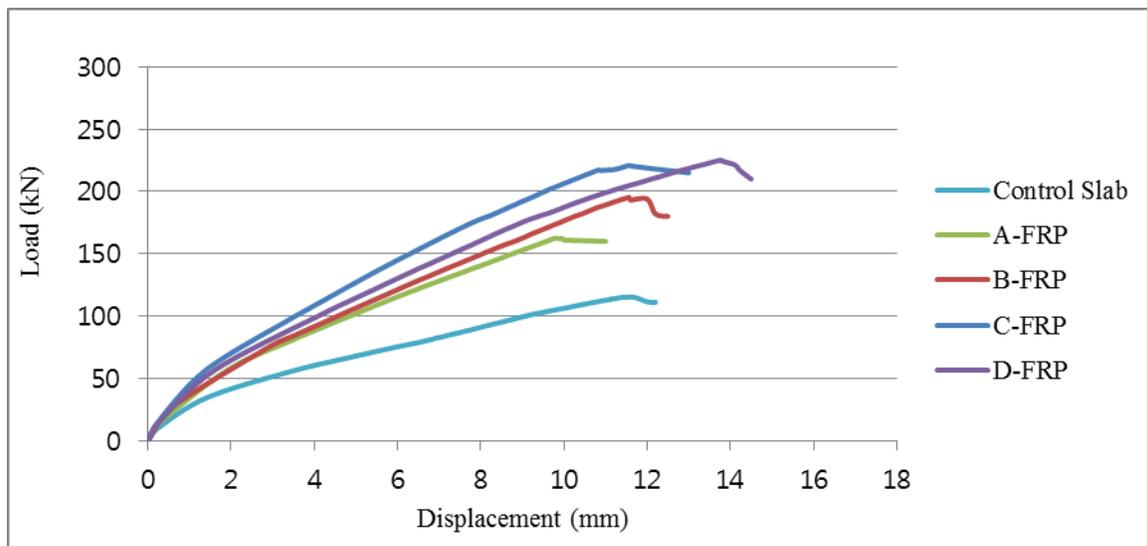
Fig. 9: Load – Displacement curves of CFRP Fan strengthening technique
