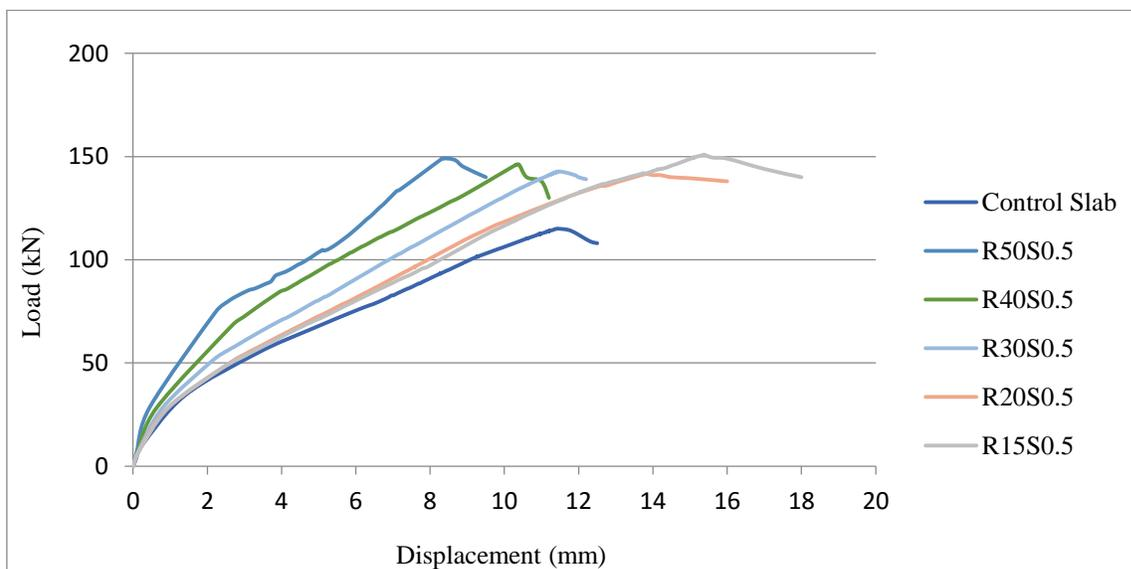
Fig 5: Load – Displacement curves of Steel Plate strengthening technique
