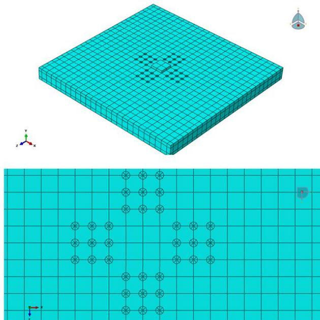
Fig. 8: Modeling of slabs strengthened by using of FRP fan technique
