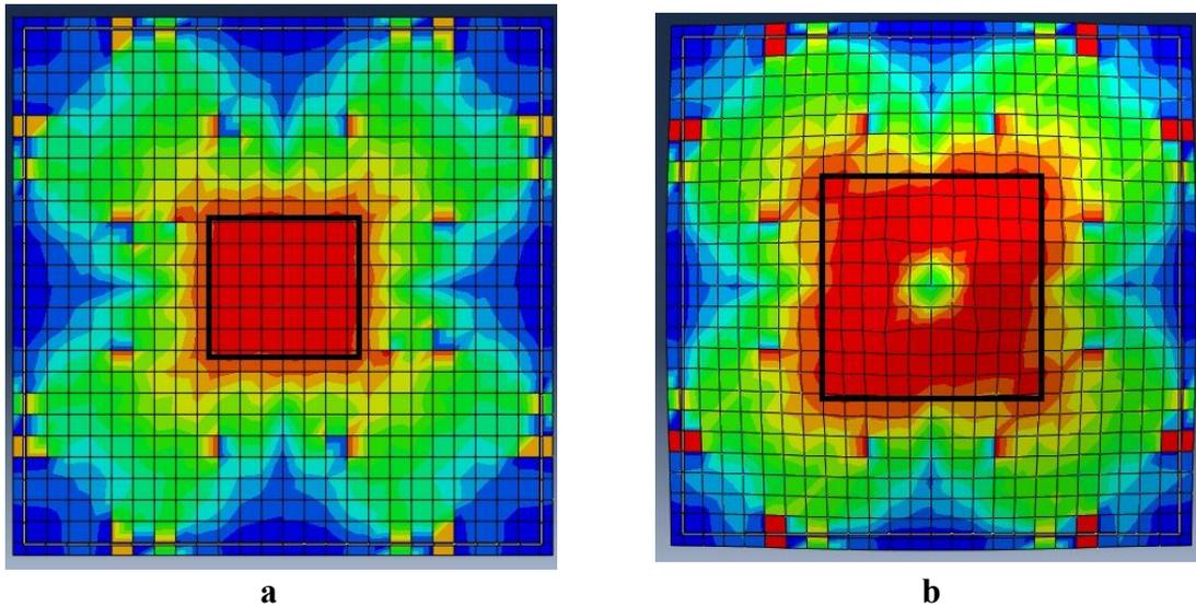
**Fig. 10: Damage parameter contour of all strengthening patterns (a: control slab, b: strengthened slab by steel sheets)**
