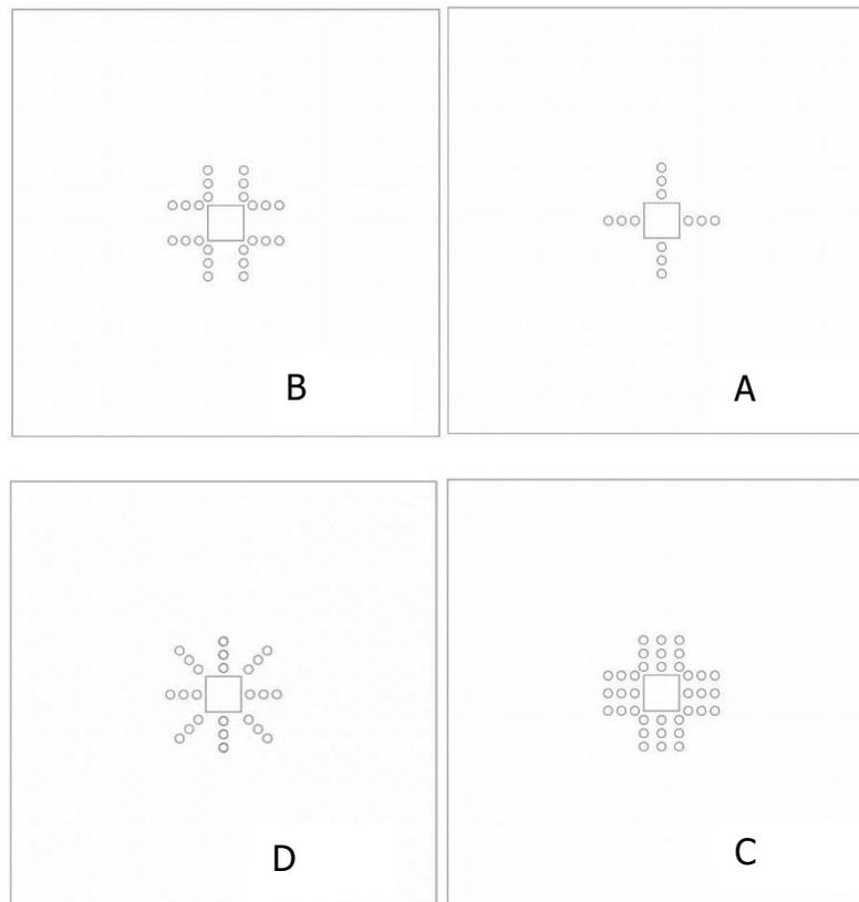
Fig. 4: Various type of FRP Fan technique
