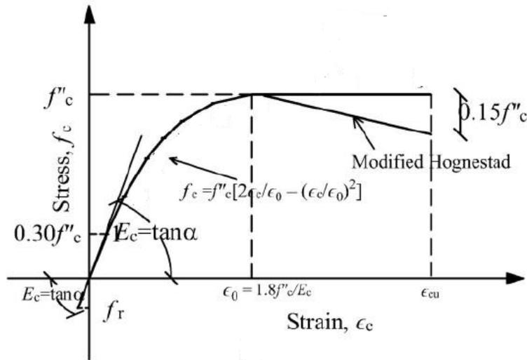
Fig. 2: Stress-strain diagram of concrete
