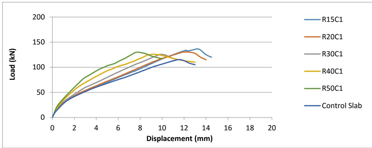
Fig 6: Load – Displacement curves of CFRP Sheet strengthening technique
