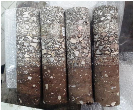
Figure 5. Individual asphalt layers of core samples in Site S05
