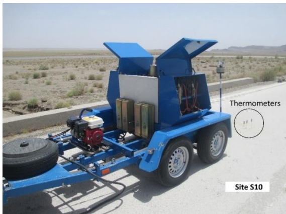
Figure 3. FWD testing and depth temperature measurements of asphalt layers
