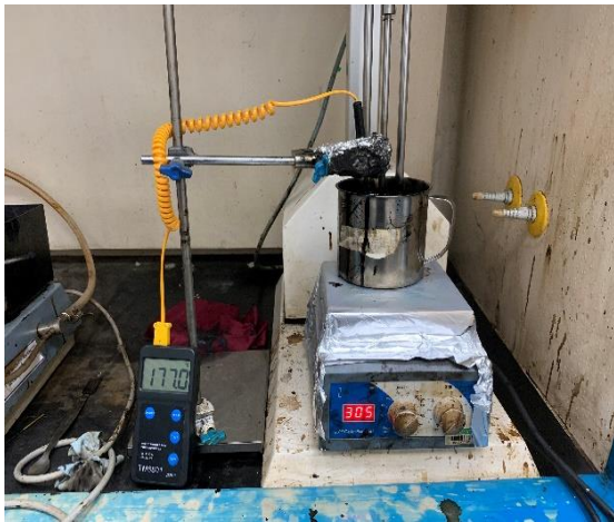
Fig. 1. The mixing process for the modified asphalt.
