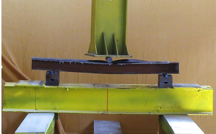
Fig. 18. Buckling of CFRP laminate covering top flange of steel beam.
