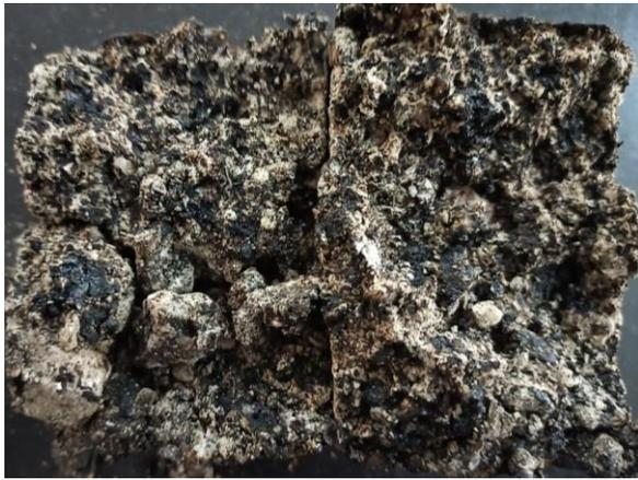
**Fig.5.** Failure patterns of RAP blends.
