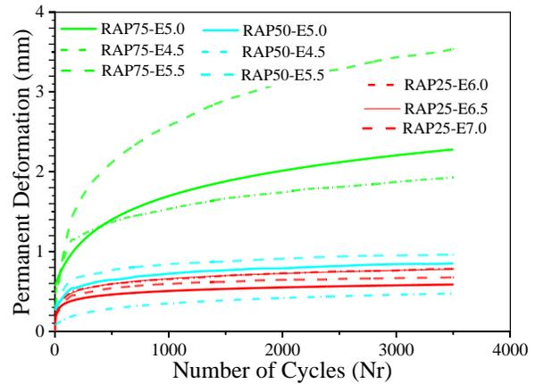
**Fig.10.** Comparison of permanent deformation curves of different RAP blends at optimum, below optimum, and above optimum emulsion contents.
