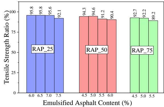
Fig. 8. Tensile strength ratio of RAP mixes.
