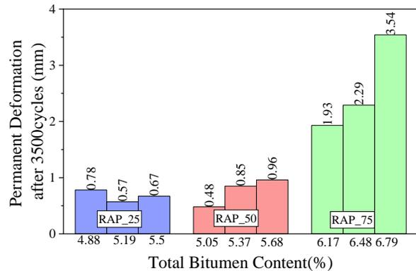
**Fig. 11** Effect of Total Bitumen Content (TBC) on Permanent Deformation.
