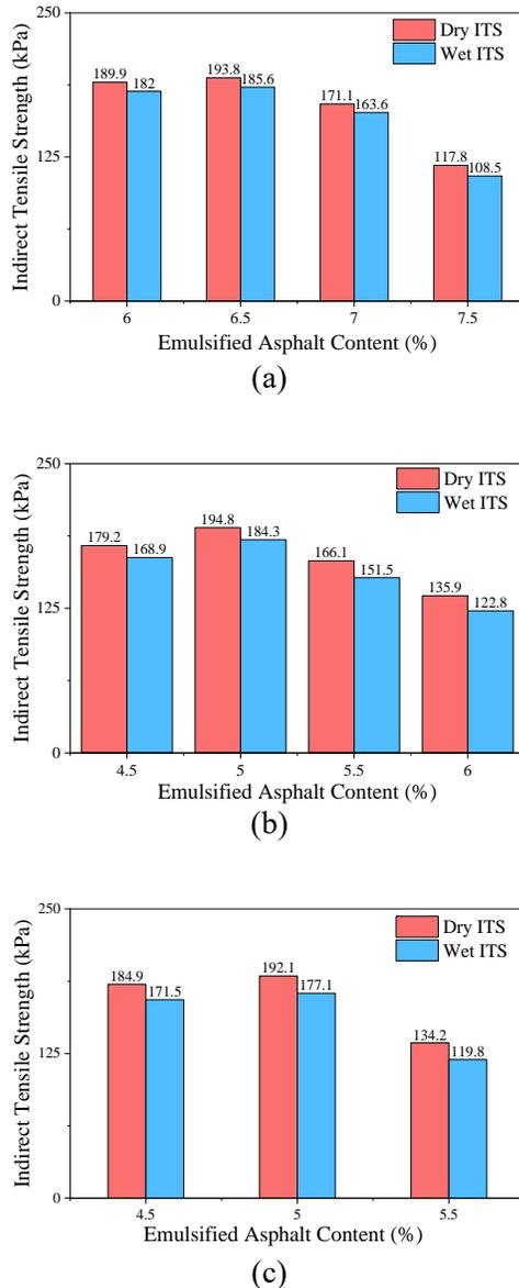
**Fig.2.** ITS test of cream for different RAP contents (a) 25% RAP (b) 50% RAP (c) 75% RAP.
