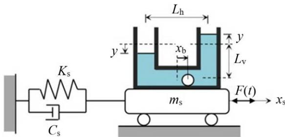
Fig. 1. 3 DOF-Model of a structure equipped with TLCBD.
