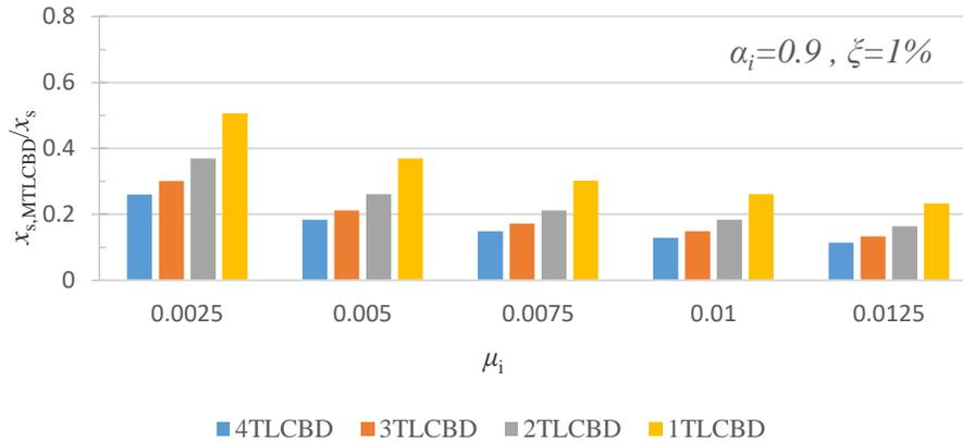
**Fig. 9.** The influence of the number of individual dampers ( $n$ ) on the response mitigation of a MTLCBD with a length ratio of  $\alpha_i = 0.9$ , in a structure with an inherent damping ratio of  $\zeta = 1\%$ .
