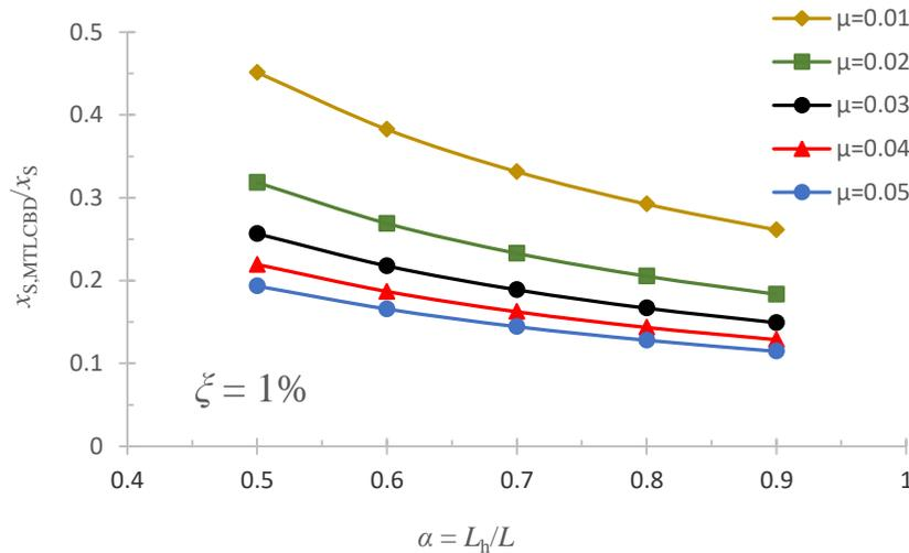
**Fig.6.** The influence of the length ratio of individual dampers,  $\alpha$ , on the response mitigation of a dual TLCBD system with various mass ratios ( $\mu$ ).
