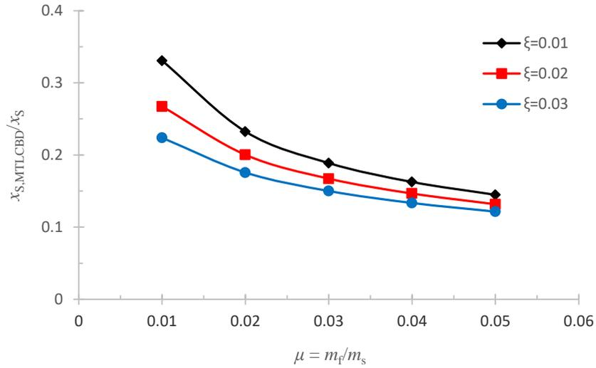
**Fig. 7.** The influence of total mass ratio ( $\mu = \sum_{i=1}^n \mu_i$ ) in response mitigation of a foursome TLCBD in which the individual dampers share the same mass ratio, and have a length ratio of  $\alpha = 0.7$ .
