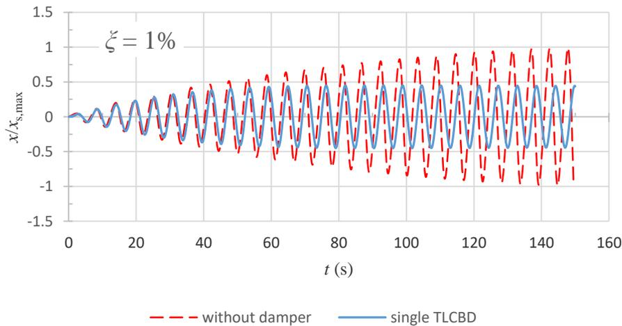
**Fig. 3.** Normalized displacement time history of the structure to a harmonic wind excitation of  $\beta = 0.99$ , a comparison between the responses of the original structure (without damper) and the structure equipped with a single TLCBD of  $\mu = 1\%$ , and  $\alpha = 0.5$ .
