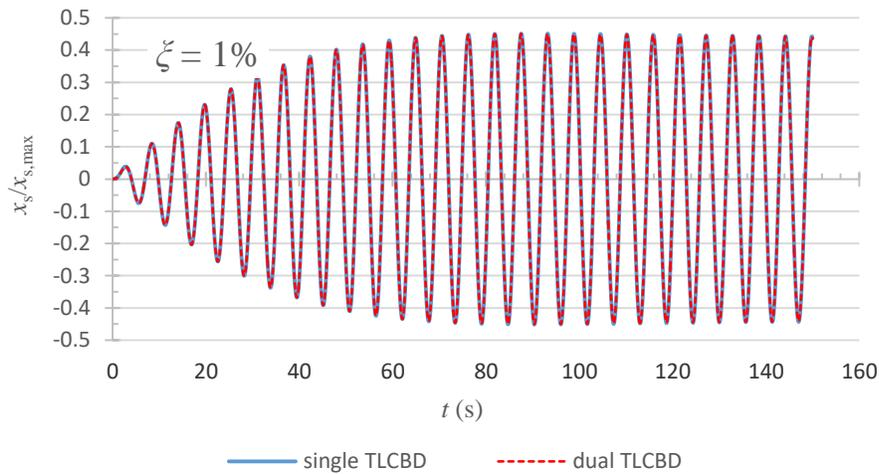
**Fig. 4.** Time history of normalized displacements in the structure equipped with a single TLCBD of  $\mu = 0.01$  and an equivalent dual TLCBD of  $\mu_i = 0.005$  ( $\alpha = 0.5$  for all dampers).
