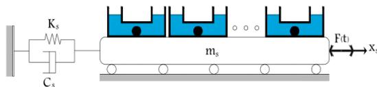
Fig. 2. A structure equipped with MTLCBD.
