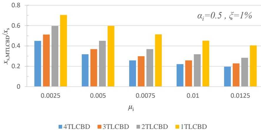
**Fig. 8.** The influence of the number of individual dampers (n) on the response mitigation of a MTLCBD with length ratio of  $\alpha_i = 0.5$ , in a structure with an inherent damping ratio of  $\zeta = 1\%$ .
