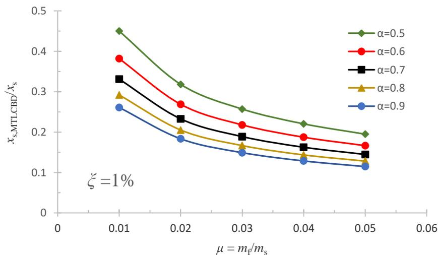
**Fig. 5.** The influence of total mass ratios,  $\mu = \sum_{i=1}^2 \mu_i$ , on response mitigation of a dual TLCBD system with various length ratios ( $\alpha$ ).
