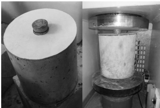
Fig. 3. DPT specimen prior to the test.
