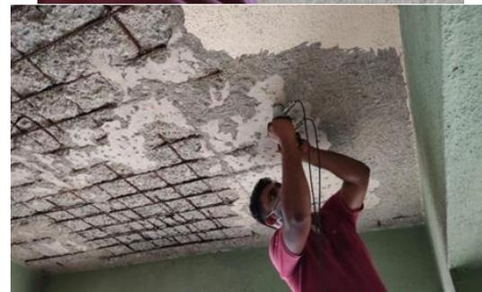
**Fig. 7.** shows building conditions currently. (NDT Testing) An ultrasonic pulse velocity test.
