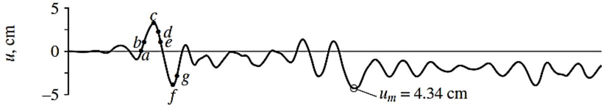
Fig. 13. Displacement response reported in [8] for the nonlinear SDOF system in example III.
