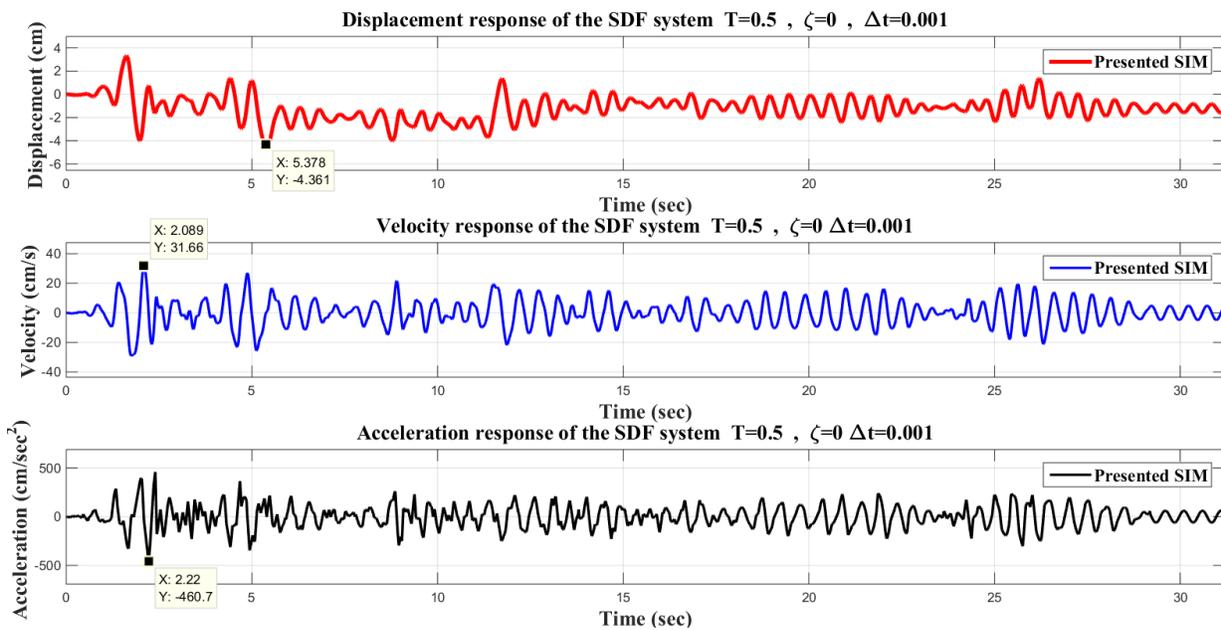
Fig. 15. Responses obtained from SIM for the nonlinear SDOF system in example III (Fine mesh).
