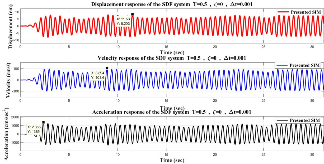
Fig. 11. Responses for the linear SDOF system in example III (Fine mesh).
