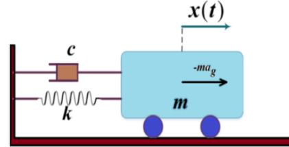
Fig. 2. Idealized mass-spring model of vibration under support excitation.
