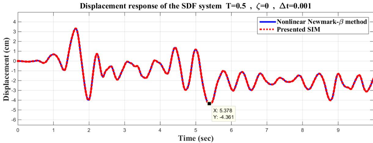
Fig. 14. Displacement response for the nonlinear SDOF system in example III.
