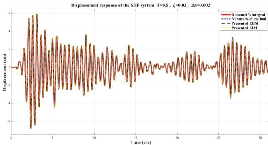
**Fig. 5.** Displacement responses for the linear SDOF system in example I (Fine mesh).
