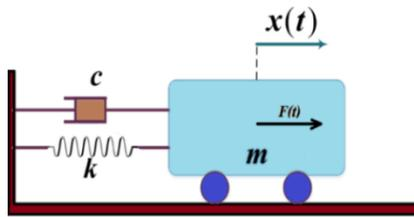
Fig. 1. Idealized mass-spring model of vibration under external force.
