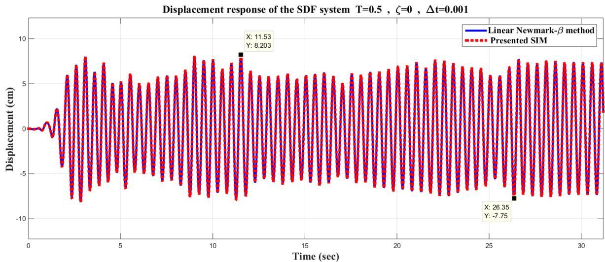
Fig. 10. Displacement response for the linear SDOF system in example III (Fine mesh).
