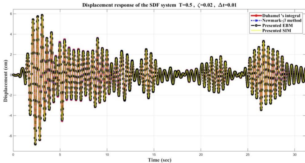
**Fig. 4.** Displacement responses for the linear SDOF system in example I (Coarse mesh).
