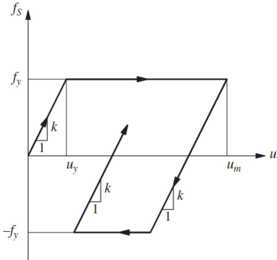
Fig. 12. Idealized elastoplastic behavior of restoring force-deformation component in example III.
