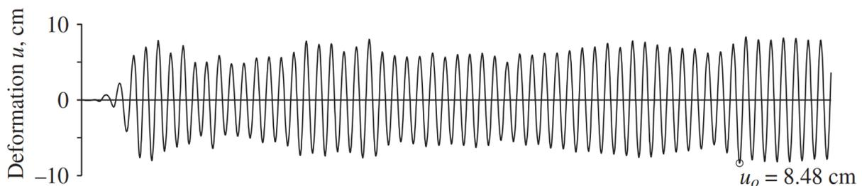
**Fig. 8.** Displacement response reported in [8] for the linear SDOF system in example III (Coarse mesh).
