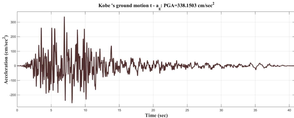
**Fig. 6.** Kobe's ground motion record.
