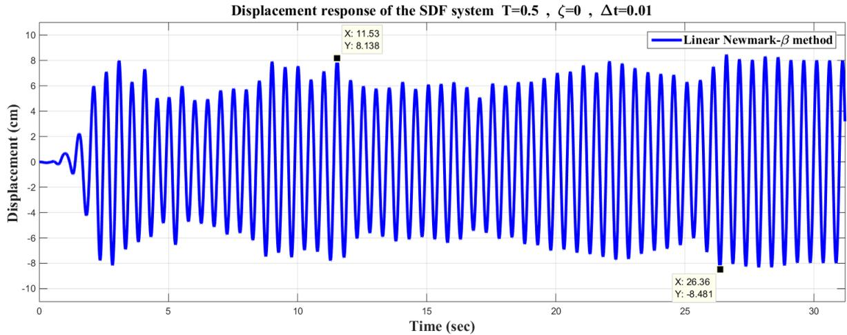
Fig. 9. Displacement response obtained from Newmark-β method for the linear SDOF system in example III (Coarse mesh).
