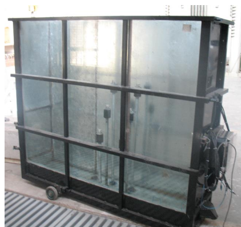
Fig. 4. A general photo of soil reservoir with soil pressure transducer and data acquisition.
