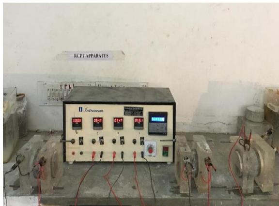
Fig. 1. Experimental test setup for RCPT test.
