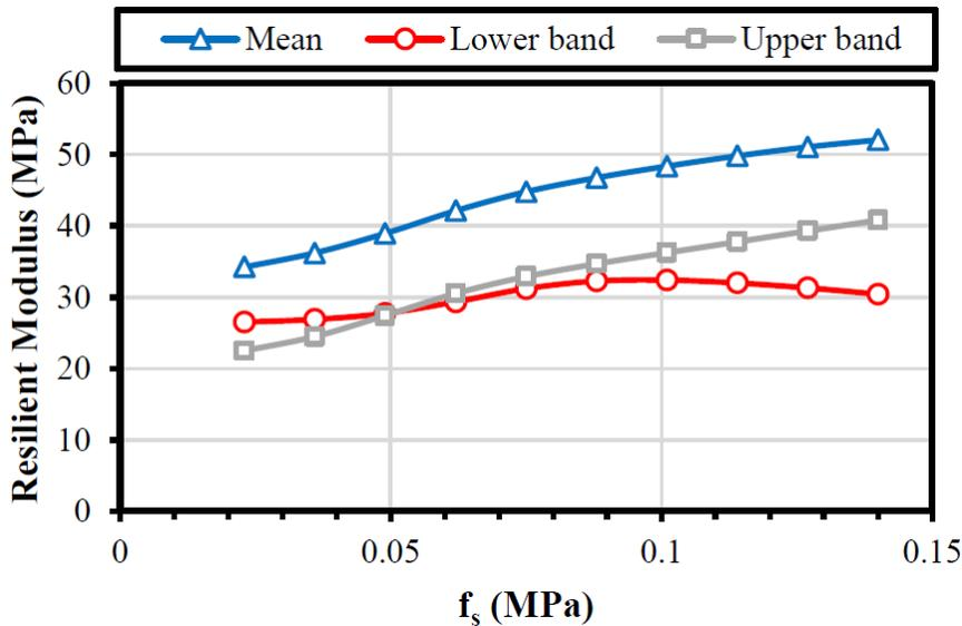
Fig. 7. The effect of sleeve friction on the resilient modulus.
