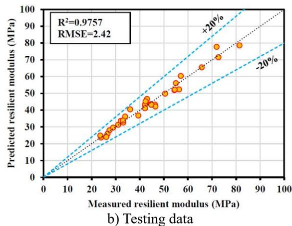
**Fig. 3.** Comparing the results of the predicted and measured resilient modulus.
