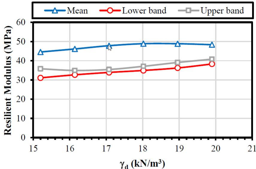
Fig. 9. The effect of the dry density of soils on the resilient modulus.
