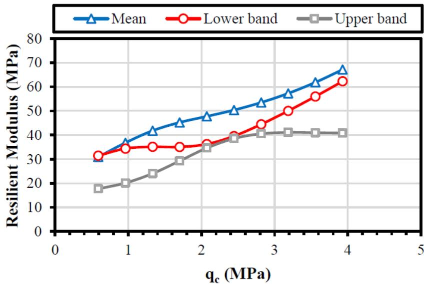
Fig. 6. The effect of the cone tip resistance on the resilient modulus.
