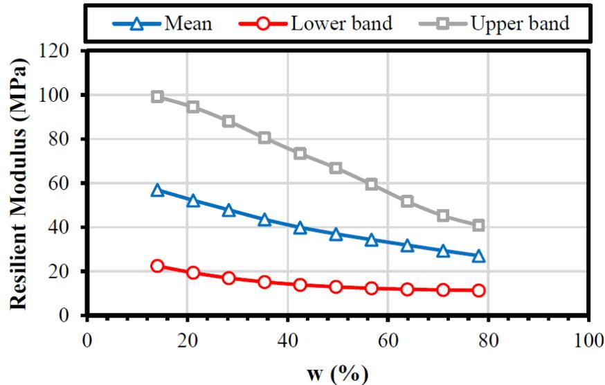
Fig. 8. The effect of moisture content of soils on the resilient modulus.
