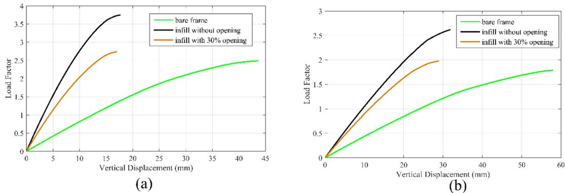
Fig 24. Vertical capacity of frame with very high importance factor (a) scenario 1 (b) scenario 2.
