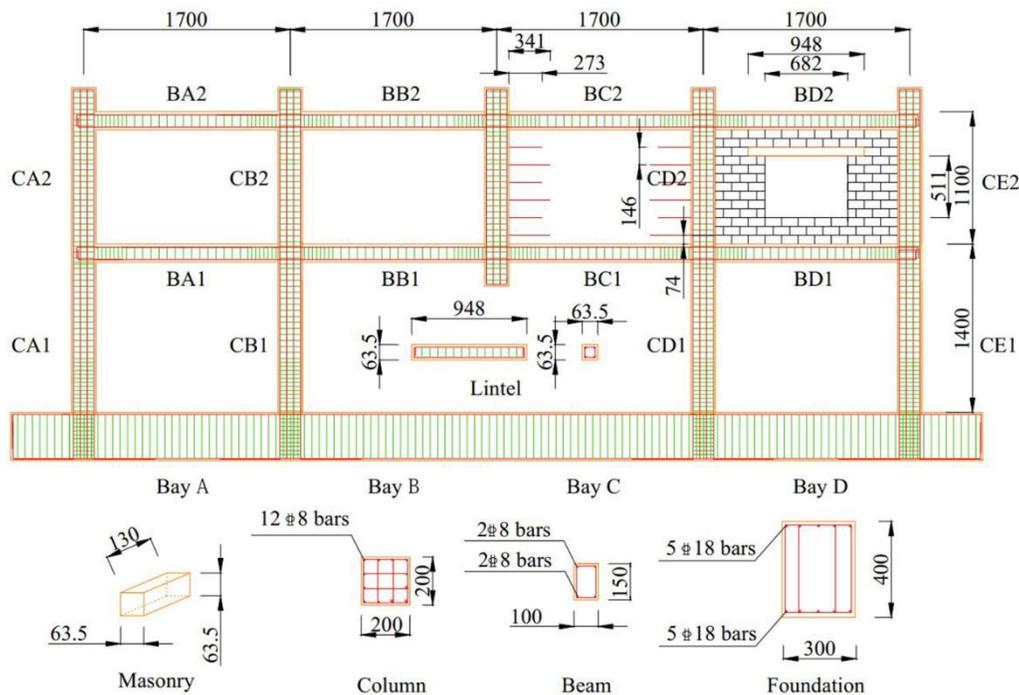
Fig 12 overall schematic and detailing of experimental research, which is conducted by Shan et al. [66].
