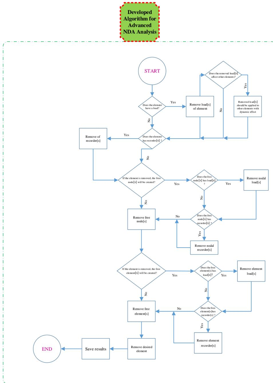
**Fig 7.** Detail of developed flowchart for element(s) removal in NDA.
