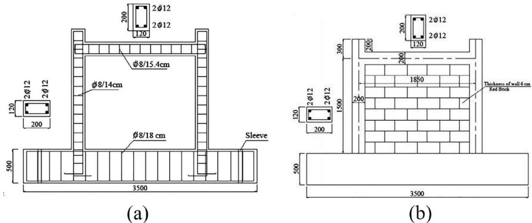
**Fig 15.** Detailing of experimental modeling (a) rebar detailing of frame (b) geometric and infill wall of frame [67].
