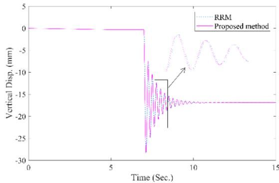
**Fig 8.** Vertical displacement of node above removed column in scenario 1 (without infill and  $IF=1.0$ ).
