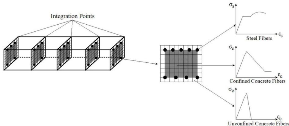
**Fig 3.** Overall considerations for each RC beam and column elements that are force based elements.
