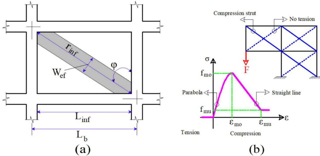
**Fig 4.** Detailing of equivalent strut compression for modeling of infill wall (a) Schematic of equivalent strut compression in an RC frame (b) Material that has been used in infill modeling.
