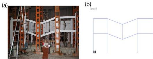
**Fig 13.** (a) Overall schematic of RC frame after column removal in experimental research [66] (b) FE modeling of RC frame that is simulated in OpenSees program.
