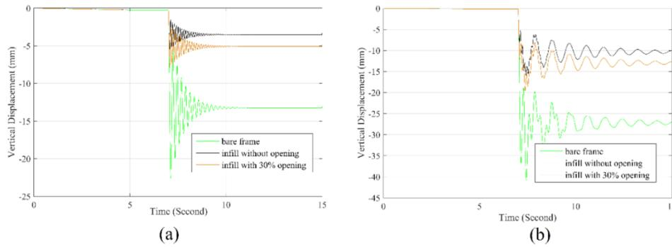
**Fig 20.** Vertical displacements corresponding to frame with very high importance factor (a) scenario1 (b) scenario 2.
