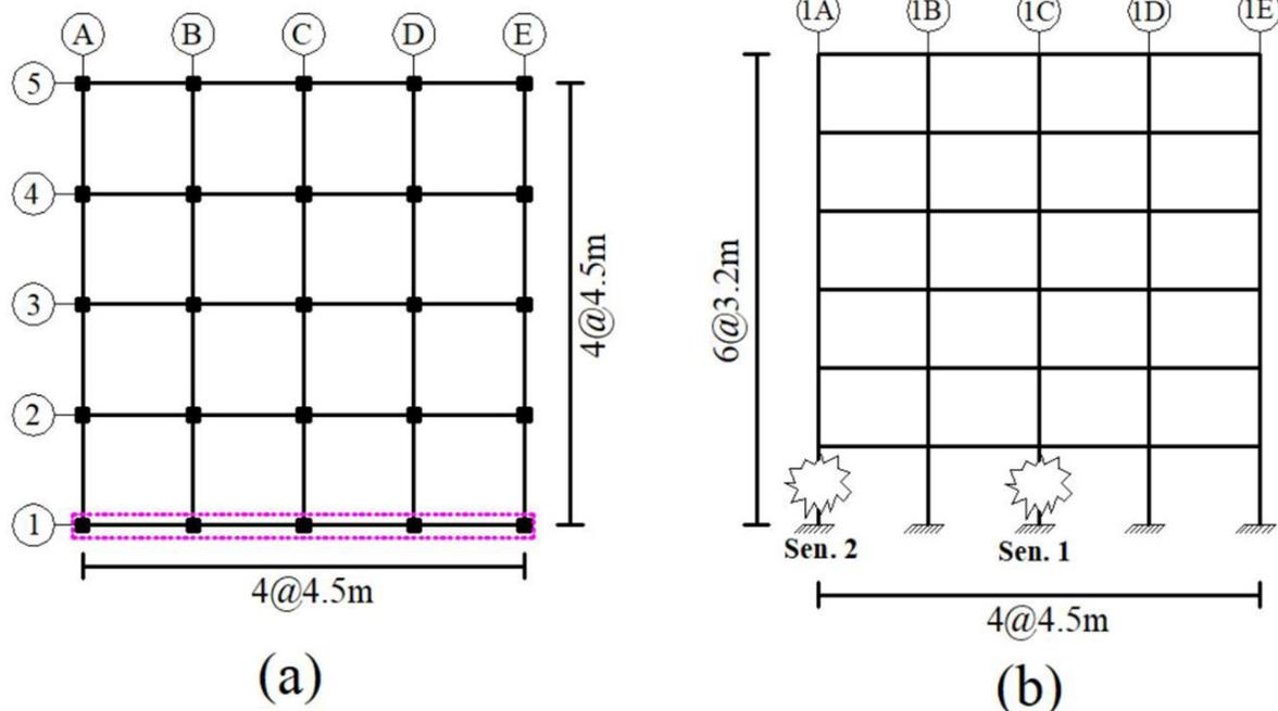
**Fig 1.** (a) Plan that been studied (b) external frame and considered scenarios for column removal.
