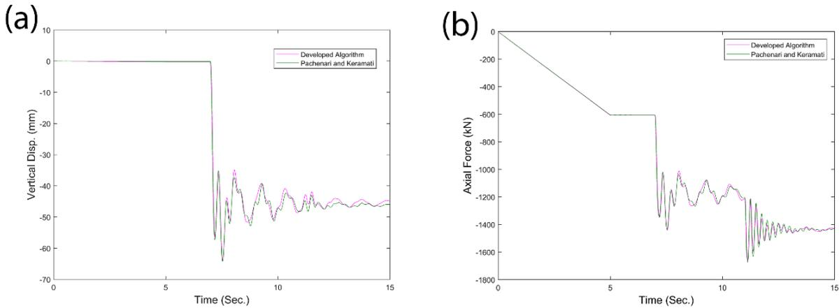
**Fig 10** comparison of developed algorithm with proposed algorithm by Pachenari and Keramati (a) vertical displacements in node  $n$  (the node above column  $i$ ) (b) axial force of column between columns  $i$  and  $j$ .
