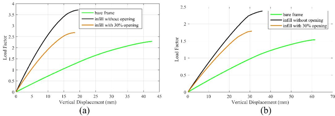
Fig 23. Vertical capacity of frame with high importance factor (a) scenario 1 (b) scenario 2.
