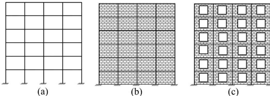
**Fig 2.** Different situation of infill walls in each frame (a) frame without infill wall (b) frame with infill wall without opening (c) frame with infill wall with 30% opening.
