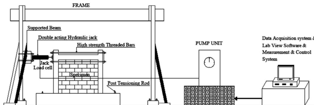
**Fig 16.** Boundary conditions and instrumentation system for the test [67].
