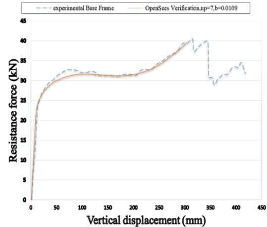
**Fig 14** Comparison of numerical and experimental results of column removal in RC frame.
