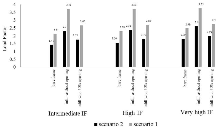
Fig 25. Chart of the maximum load factor in different stages of infill wall and importance factor levels.
