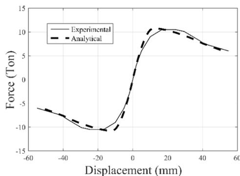
**Fig 17.** Comparison between push hysteretic in analytical and experimental results.
