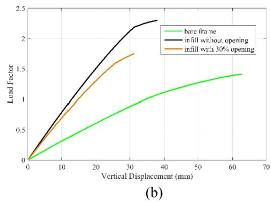
**Fig 22.** Vertical capacity of frame with intermediate importance factor (a) scenario 1 (b) scenario 2.
