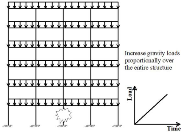
Fig 11. Overall schematic of PDA.
