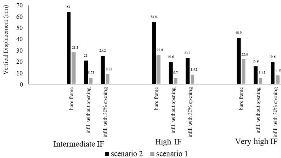
**Fig 21.** Chart of the vertical displacement in different stages of infill wall and importance factor levels.
