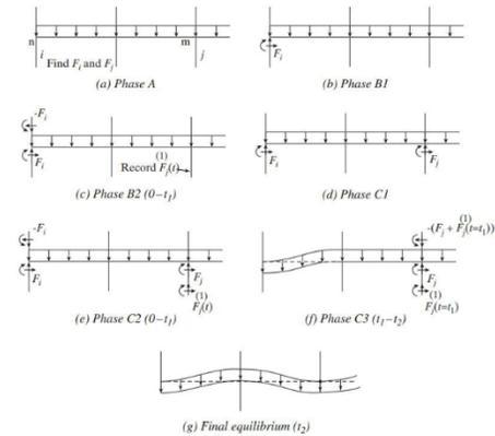
**Fig 9.** Proposed method for two-column removal in successive manner by Pachenari and Keramati [60].
